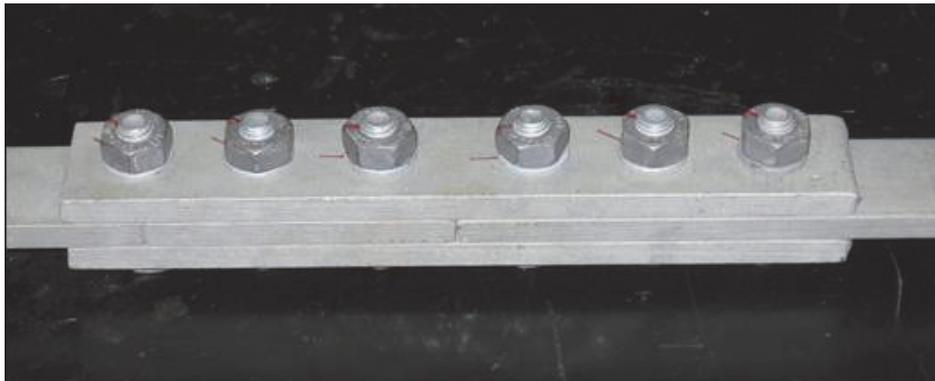
Figure 2: Hot-dip galvanized bolted connection before the test.
