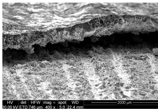
Figure 6: Layer thickness from a SEM image.
