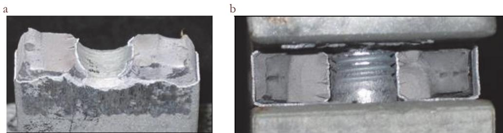
Figure 5: Typical fracture surface after cyclic loading. (a) Plate and (b) bolted part.
