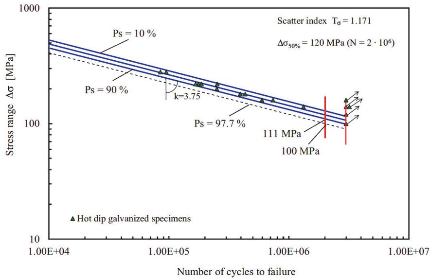
Figure 7: S-N-curves of hot dip galvanized connections.
