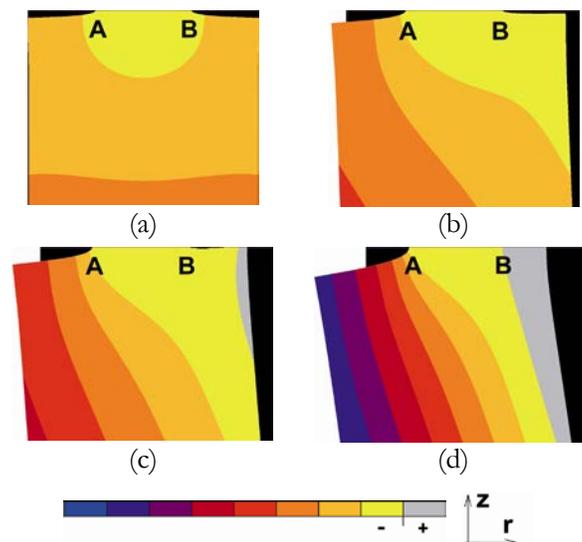
Figure 5: Displacement  $u_z$  for  $d/D=0.4$ : (a)  $\varepsilon/D=0$ ; (b)  $\varepsilon/D=0.025$ ; (c)  $\varepsilon/D=0.050$ ; (d)  $\varepsilon/D=0.125$ .
