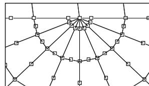
Figure 2: Detail of the finite element mesh in the vicinity of the crack tip.
