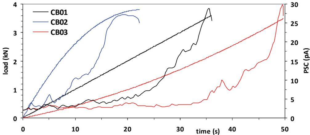
Figure 2: The time variation of the applied 3PB load and the corresponding time variation of the PSC, during all three experiments conducted.
