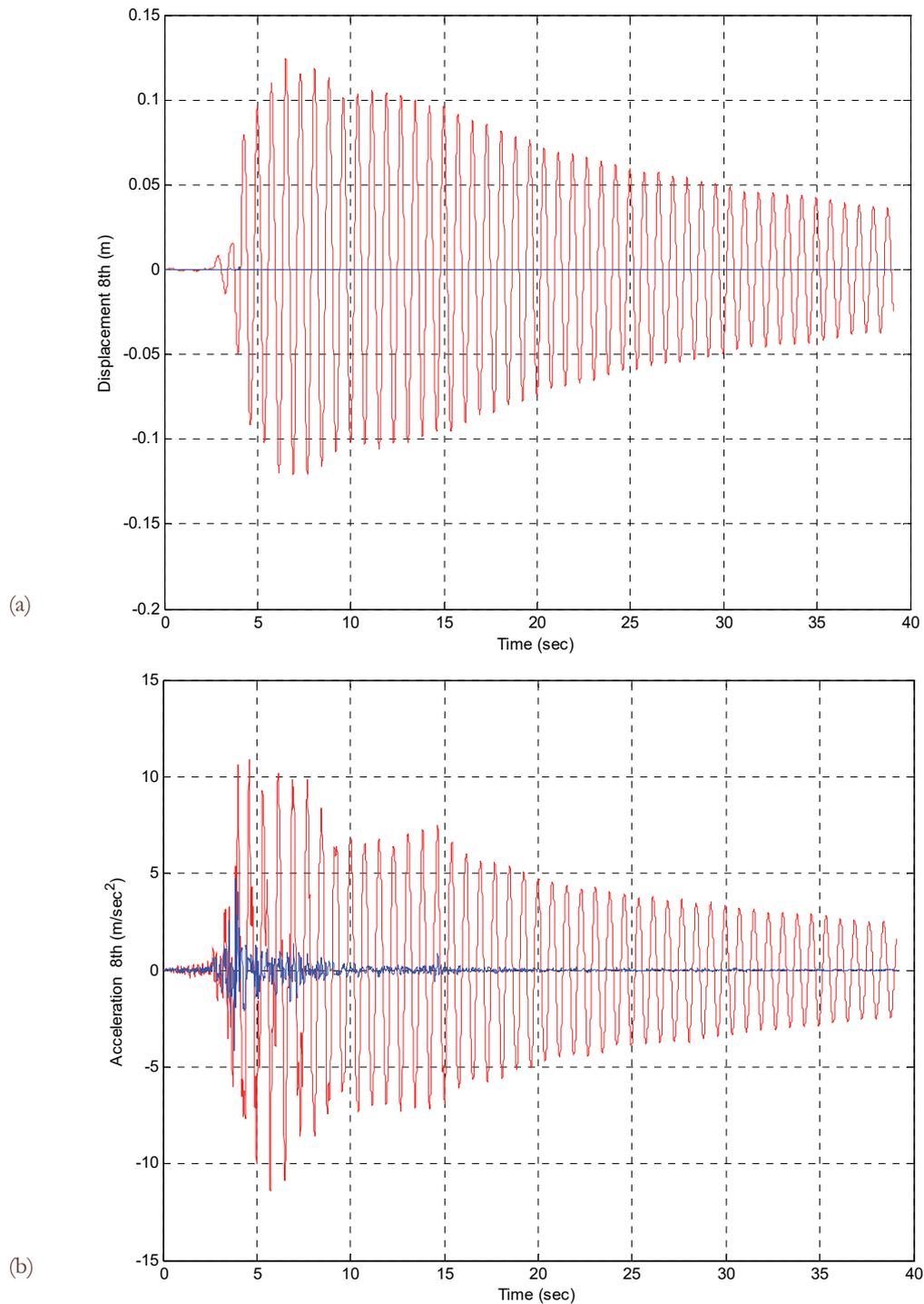
Figure 4: Displacement and the acceleration from 8<sup>th</sup> floor for the controlled and uncontrolled structure.
