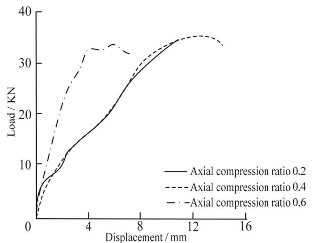
Figure 12: Curves of load-displacement (corrosion rate 2%).
