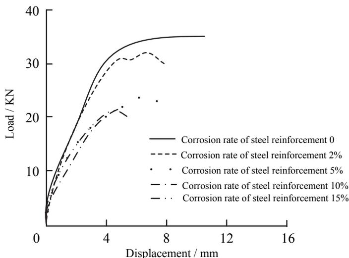
Figure 10: Curves of load-displacement (axial compression ratio 0.6).
