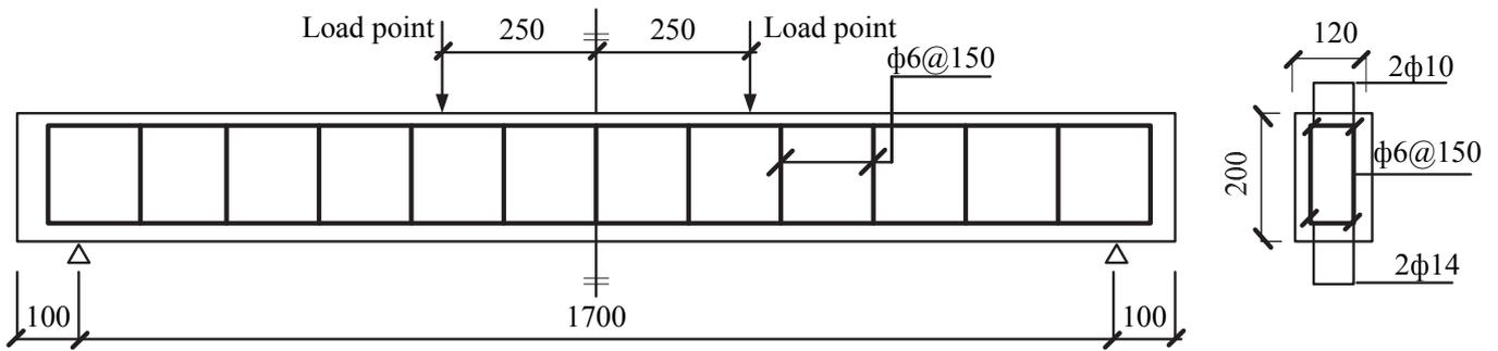
Figure 3: Size of test beam and reinforcement
