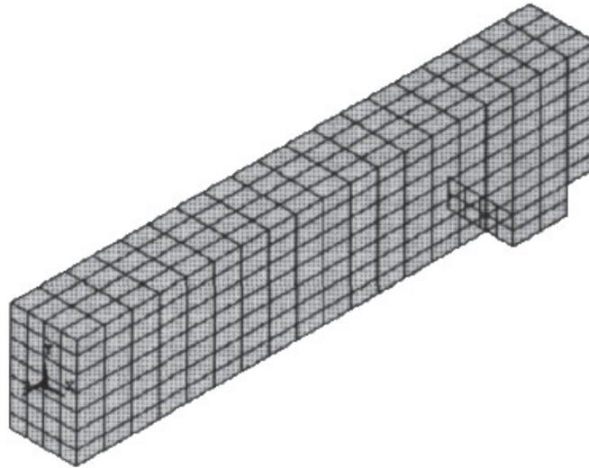
Figure 5: Grid generation of concrete unit.
