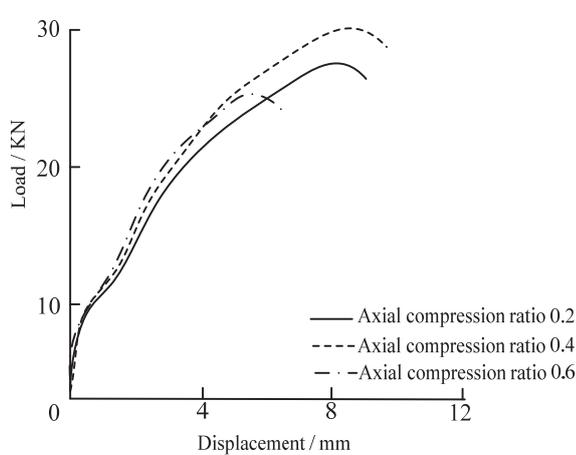
Figure 13: Curves of load-displacement (corrosion rate 5%).
