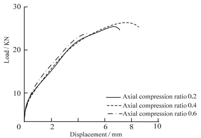
Figure 14: Curves of load-displacement (corrosion rate 10%).
