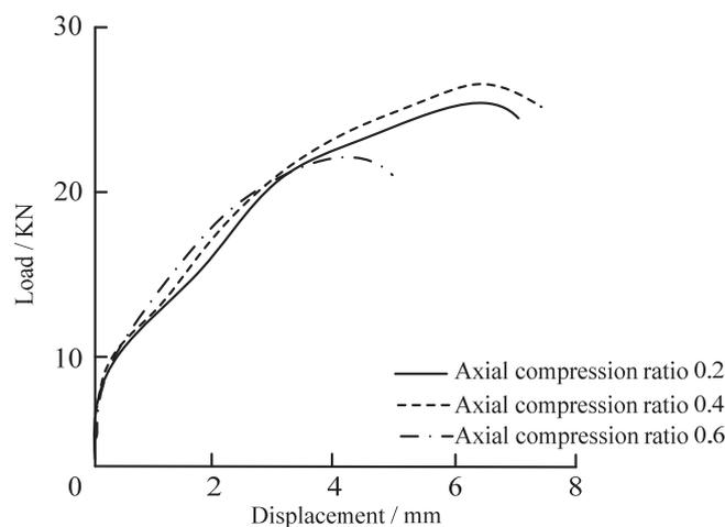
Figure 15: Curves of load-displacement (corrosion rate 15%).
