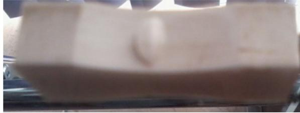
Figure 8: Bubble or protuberance at the specimen neck section, under ultrasonic fatigue testing (before crack propagation).
