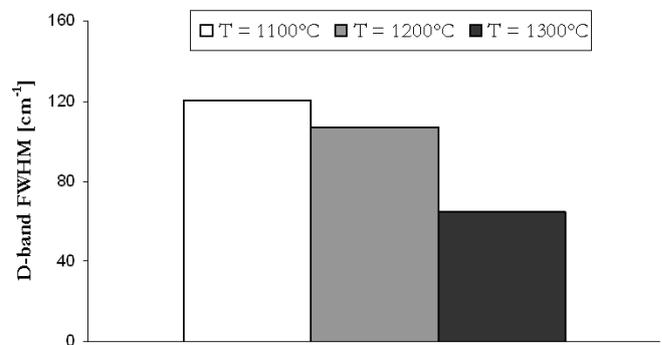
Figure 5: Full width at half maximum (FWHM) of the D band of Py-C deposited at 1100, 1200 and 1300 °C.
