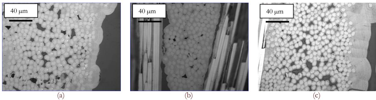
Figure 8: Optical micrographs the  $C_f/C$  cross sections at (a) 1100 °C, (b) 1200 °C and (c) 1300 °C.
