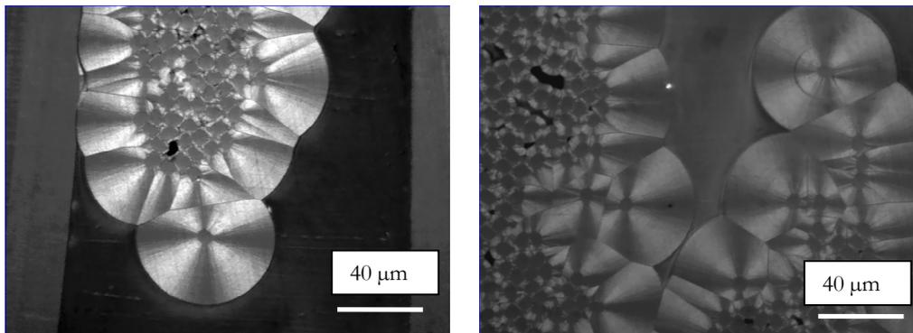
Figure 2: PLM micrographs of Py-C deposited around the carbon fibres at 1300 °C.
