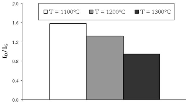
Figure 4: Intensity ratio of D and G bands of Py-C deposited at 1100, 1200 and 1300 °C.
