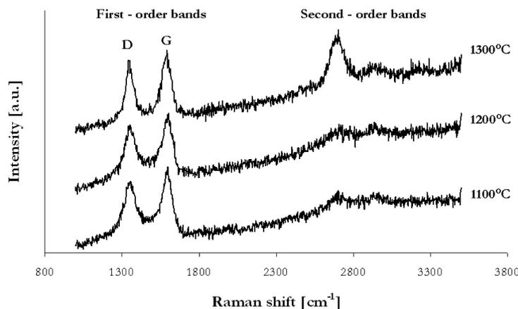
Figure 3: Raman spectra of Py-C deposited at 1100, 1200 and 1300 °C.
