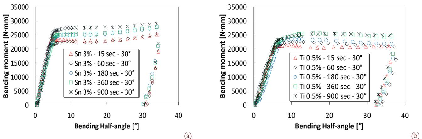
Figure 4: Bending behavior of galvanized specimens: a) galvanized in Zn-Sn bath, b) galvanized in Zn-Ti bath.
