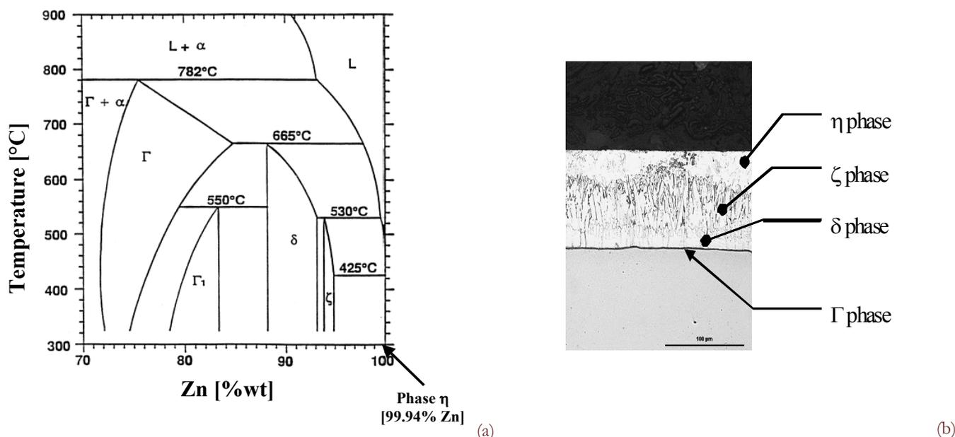
Figure 1: Intermetallic phases in a traditional hot dip galvanizing coating: a) Zn-Fe status diagram portion [1], b) Morphological aspects of intermetallic phases.
