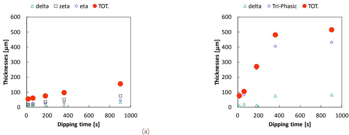
Figure 3: Coatings and their intermetallic phases thicknesses: a) coatings from Zn-Sn bath, b) coatings from Zn-Ti baths.
