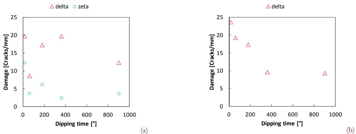
Figure 7: Intermetallic phases radial damage: a) in Zn-Sn coatings, b) in Zn-Ti coatings.
