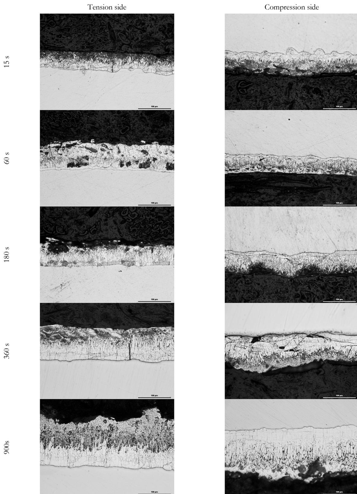
Figure 5: LOM analysis of intermetallic phases damage in Zn-Sn coatings.
