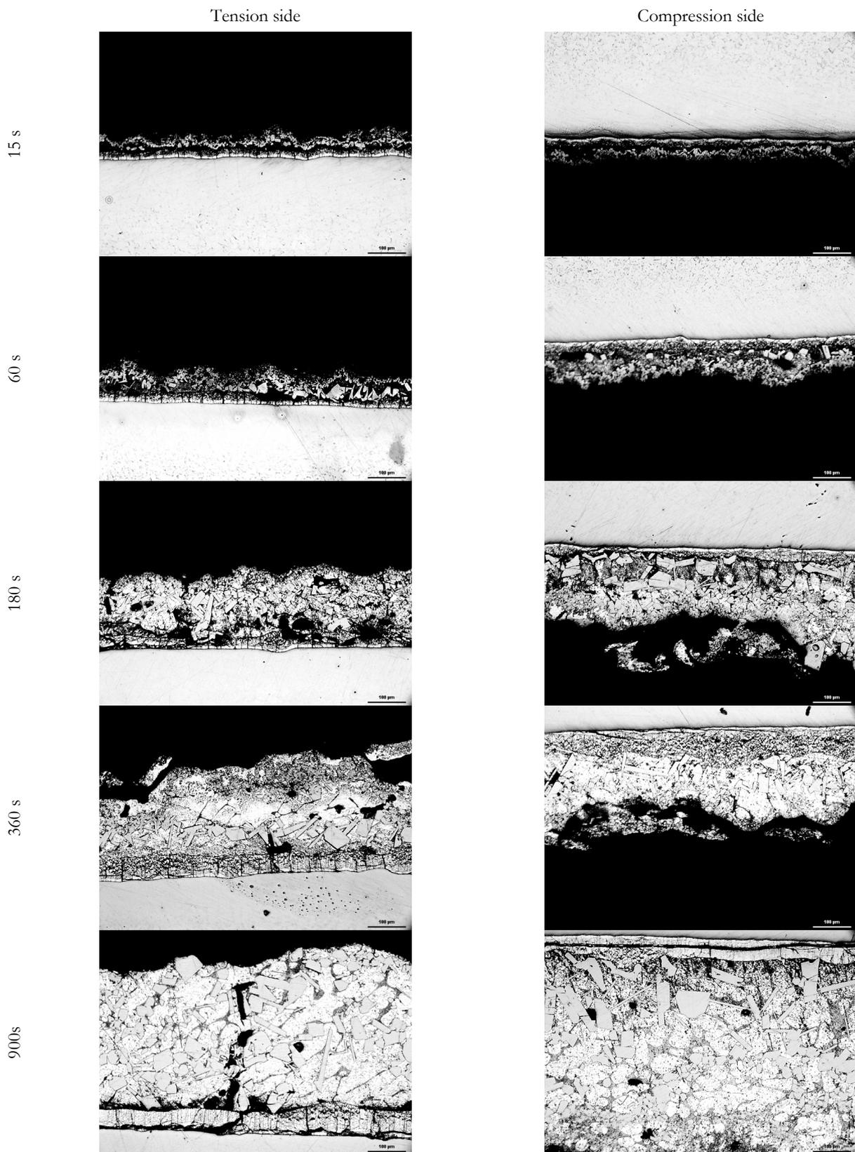
Figure 6: LOM analysis of intermetallic phases damage in Zn-Ti coatings.
