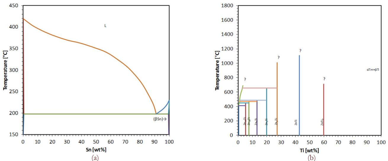
Figure 2: Equilibrium phases diagrams [11]: a) Zn-Sn alloys, b) Zn-Ti alloys.
