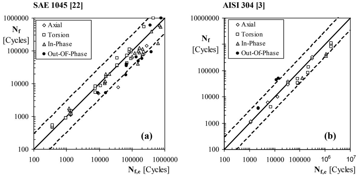
**Figure 5:** Estimated,  $N_{f,e}$ , vs. experimental,  $N_f$ , fatigue life diagrams for specimens made of SAE 1045 [22] (a) and AISI 304 [3] (b).
