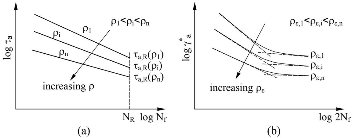
**Figure 1:** Modified Wöhler curves (a) and modified Manson-Coffin curves (b).
