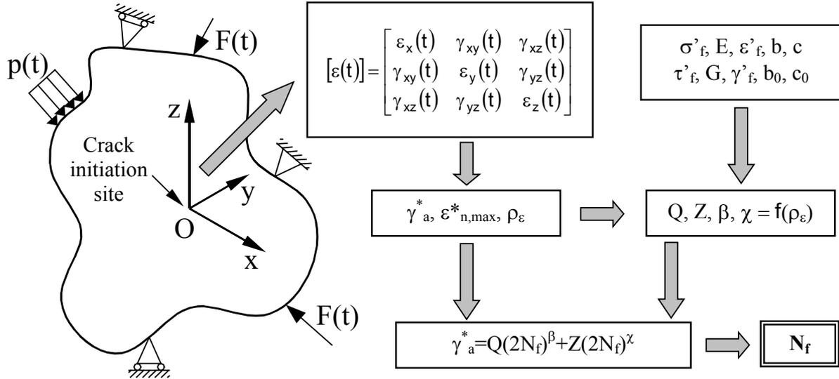
**Figure 4:** Procedure to apply the Modified Manson-Coffin curve method.
