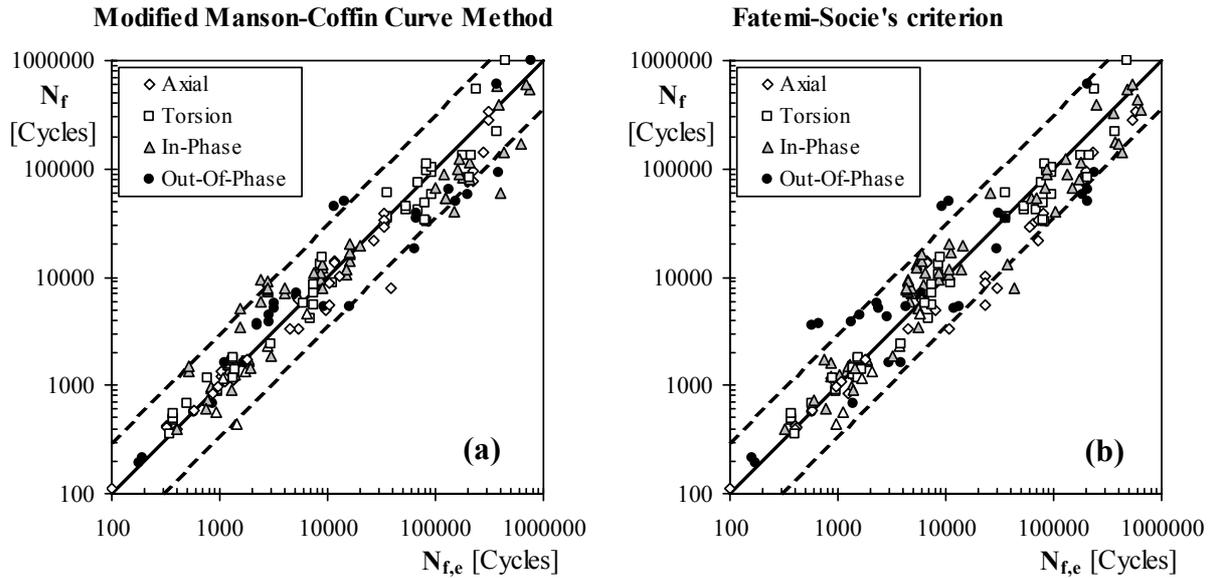
**Figure 6:** Estimated,  $N_{f,e}$ , vs. experimental,  $N_f$ , fatigue life diagrams obtained applying both the Modified Manson-Coffin curve method (a) and Fatemi-Socie's criterion [26] (b).
