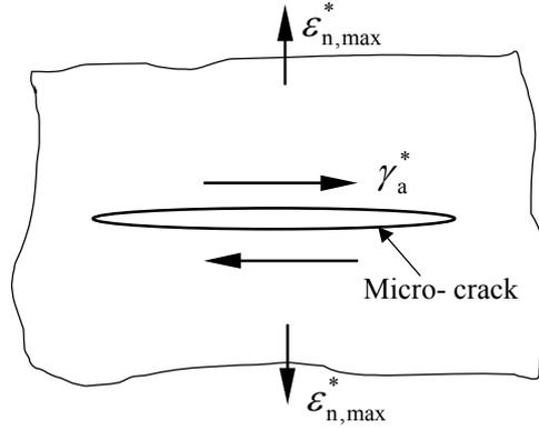
**Figure 2:** Fatigue Damage Model.
