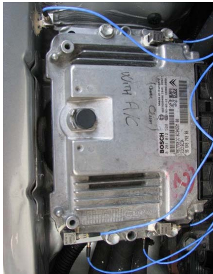
Figure 3: Vibration measurement by piezo transducers (Ver.1)
