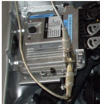
Figure 5: Vibration measurement by one-axis inductive sensors (Ver.1)
