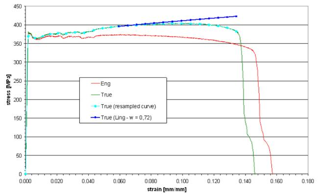
Figure 9: Comparison among Yun Ling method and experimental data in terms of stress-strain curves.
