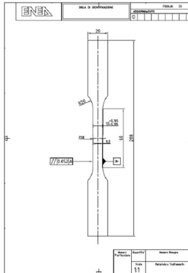
Figure 1: Geometry of the samples.
