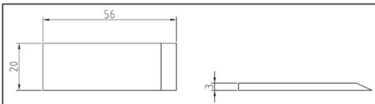
Figure 2: Geometry of the aluminum tabs.
