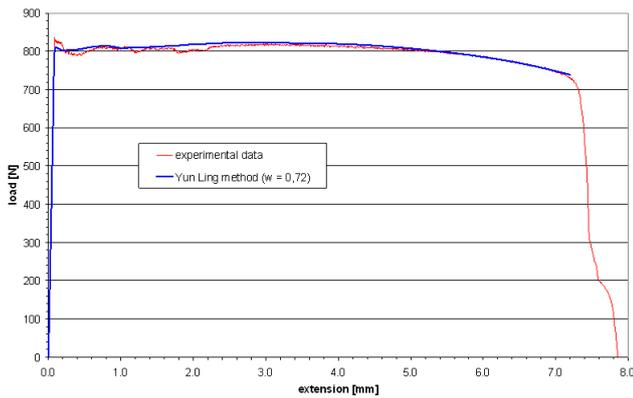
Figure 8: Calibration of the Yun Ling method vs. experimental data in terms of load-extension curves.
