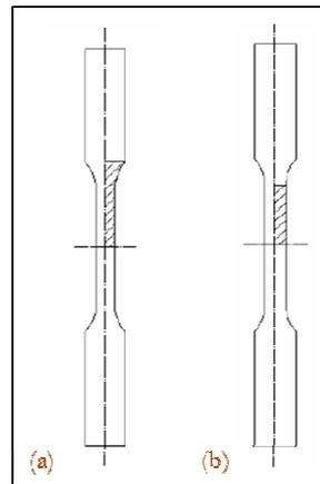
Figure 5: Simplified model for the sample: a) part subjected to tensile stress b) part instrumented by the extensometer.
