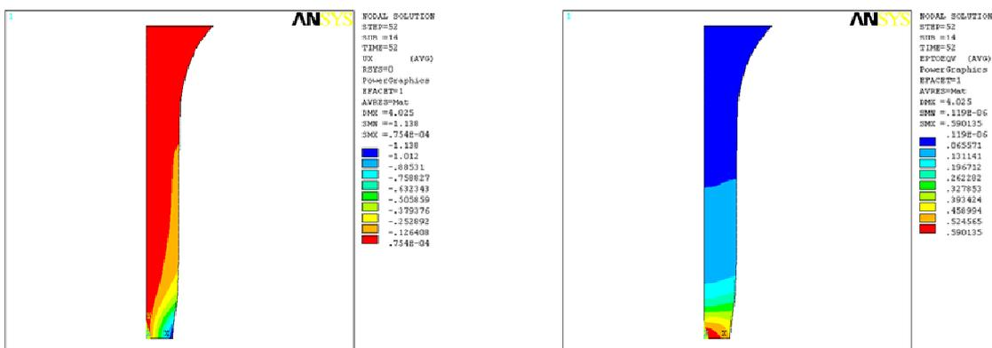
Figure 7: Distribution of transversal displacements (left image) and strain (right image) on the examined part a).
