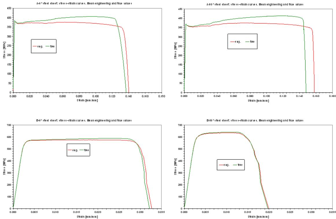
Figure 4: Comparison between engineering and true  $\sigma$ - $\epsilon$  curves
