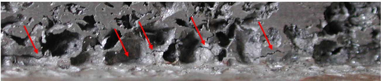
Figure 4: Fatigue failure at the interface core-skin
