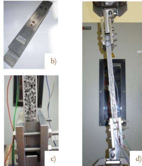
Figure 1: a) Specimens used in the testing program and results; b) Type of specimen tested; c) Clamping method; d) Specimen loaded in test machine.
