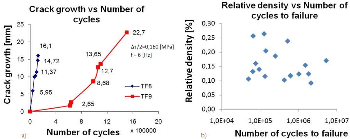
Figure 3: a) Crack growth for two specimens at the same load conditions; b) Relative density vs Number of cycles
