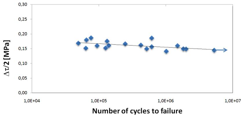
Figure 2: Shear fatigue curve for AFS.
