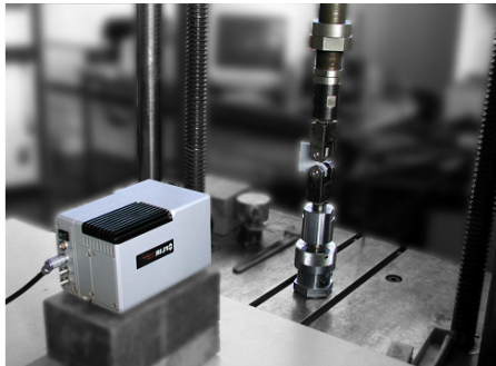
Figure 1: Thermo-camera with CT specimen.
