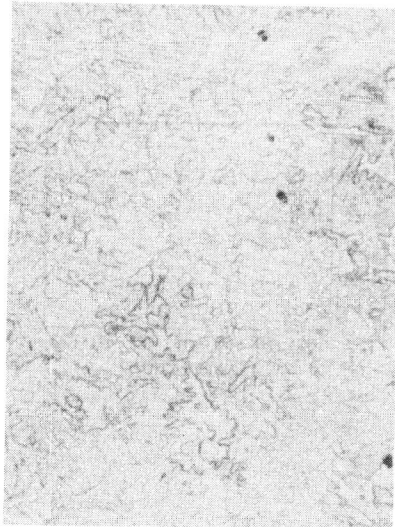
Figure 7: Unreheated CGHAZ, PWHT condition. Magnification: 300×
