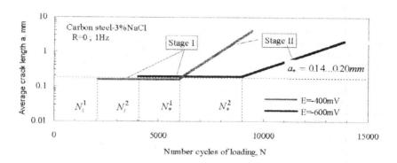
Figure 3 Average crack length versus number cycles of loading under different electrochemical conditions on the notch surface.
