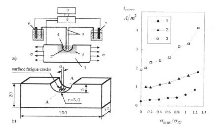
Figure 1 Principal scheme of tests (a) and Figure 2 Dependencies of corrosion specimen geometry (b): 1 - specimen, 2 - current density  $i_{corr}$  on the ratio semicircular notch; 3 - protective film; 4 corrosive environment; 5 - electrolytic capillaries; 6 - reference electrode; 7 auxiliary electrode; 8 - potentiostat; 9 - XY recorder.
