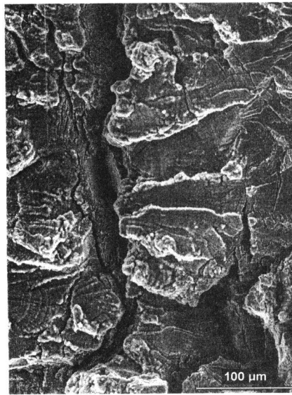
Fig. 9: EAC- pre-fatigue interface, EnvIII. Fig. 10: Detail of Fig9., EnvIII, 23 \mu m/h.
