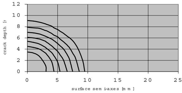
Figure 8. Cyclic Tension Surface Crack Shapes ( Base Metal ).
