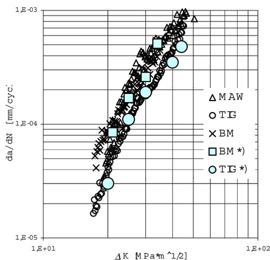
Figure 2. Type 2 specimen crack growth rate results in as welded condition ( designation \* ) stands for surface cracks ).
