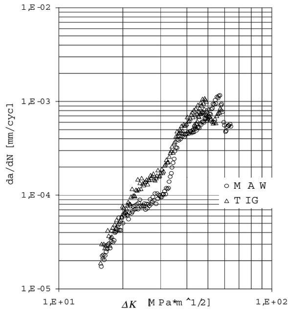
Figure 4. Type 3 specimen crack growth rate results in as-deposited condition.
