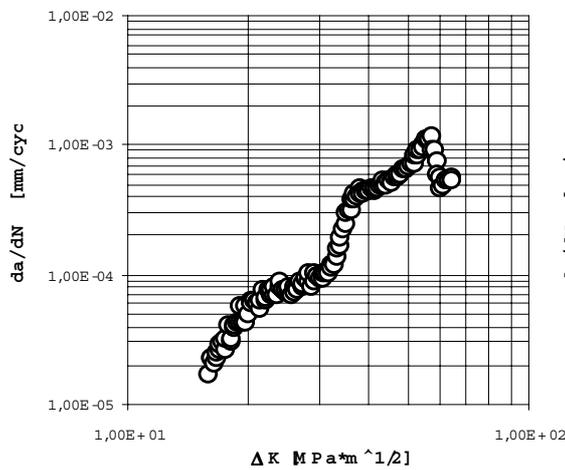
Figure 6. Fatigue crack growth rate data for TYPE 3 test specimen in as-deposited condition.
