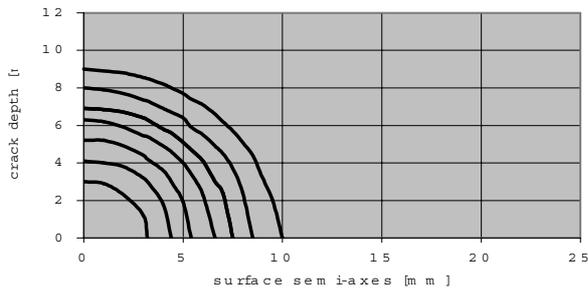
Figure 9. Cyclic Tension Surface Crack Shapes ( Weld Metal ).
