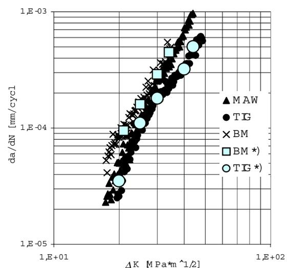
Figure 3. Type 2 specimen crack growth rate results after heat treatment ( designation \* ) stands for surface cracks ).
