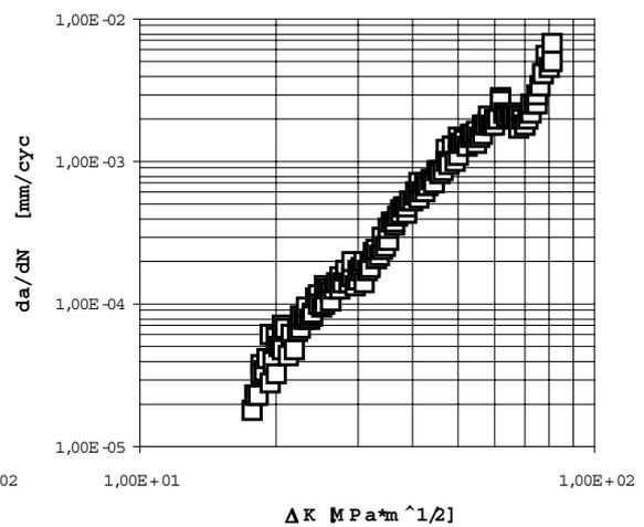
Figure 7. Fatigue crack growth rate data for TYPE 3 test specimen after heat treatment.
