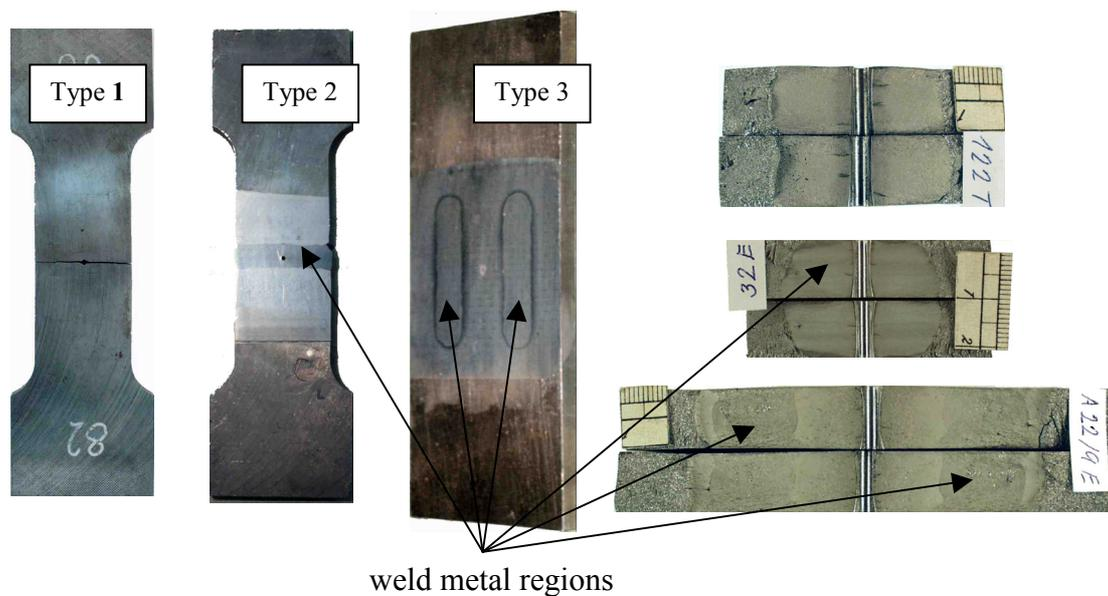
Figure 1. TYPE 1, TYPE 2 and TYPE 3 CCT test specimens.
