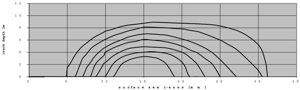
Figure 10. Cyclic Tension Surface Crack Shapes
