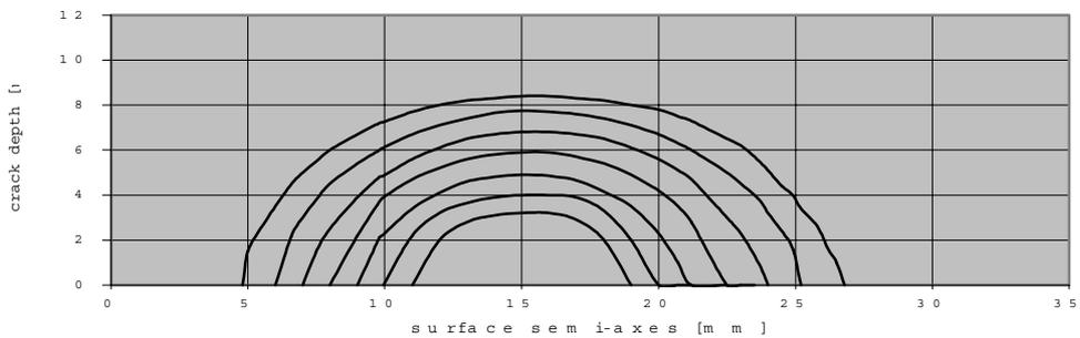
Figure 11. Cyclic Tension Surface Crack Growth Shapes
