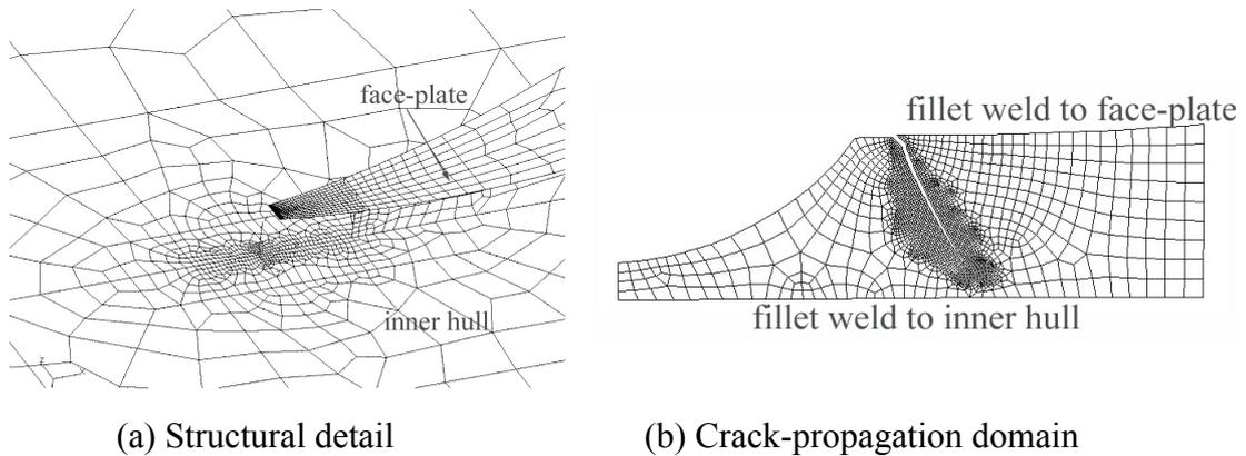
Figure 4. Critical detail at the end of a horizontal girder: (a) a super-element surrounding the crack-propagating domain, (b) an automatically generated FE-model of the crack-propagating domain.
