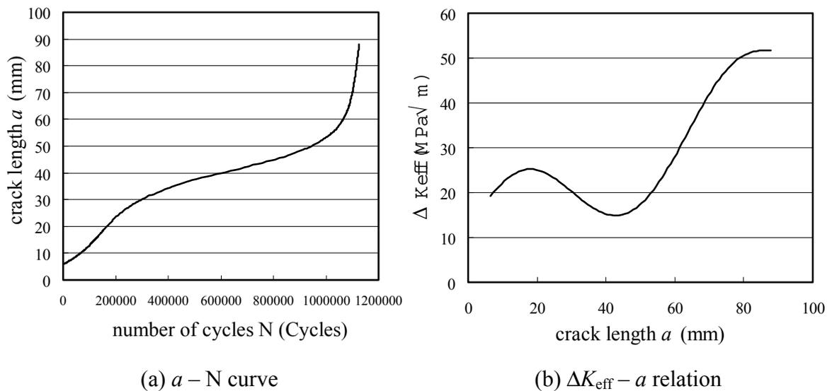
Figure 5. Simulated fatigue crack growth and the corresponding stress intensity range.
