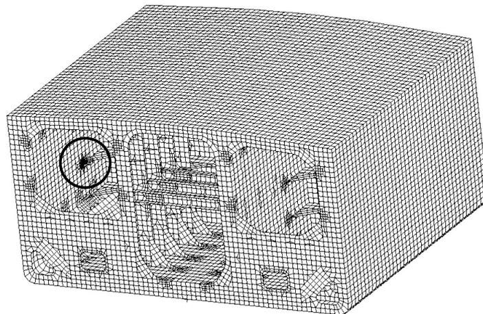
Figure 3. Critical location of fatigue damage of a double hull tanker: FE-model of a unit hull module.
