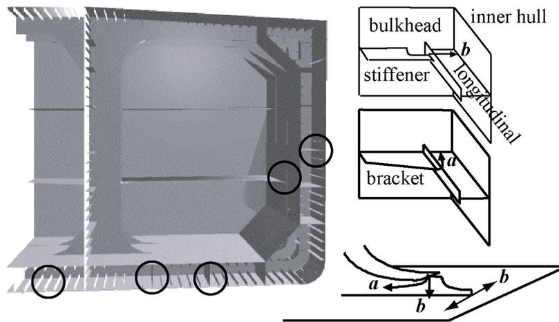
Figure 1. Typical fatigue cracks in ship structures, where cracks of type (b) should be prevented.
