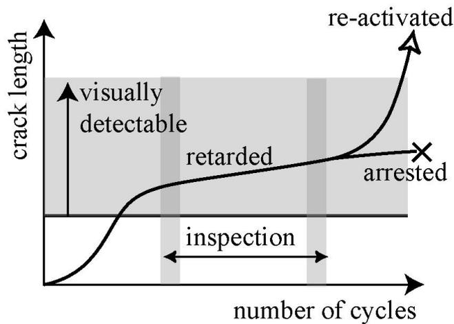
Figure 2. Concept of fatigue control of a ship structure.
