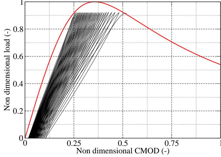
Figure 2. Load vs. CMOD for case  $\frac{P_{upper}}{P_{peak}} = 0.92$ .
