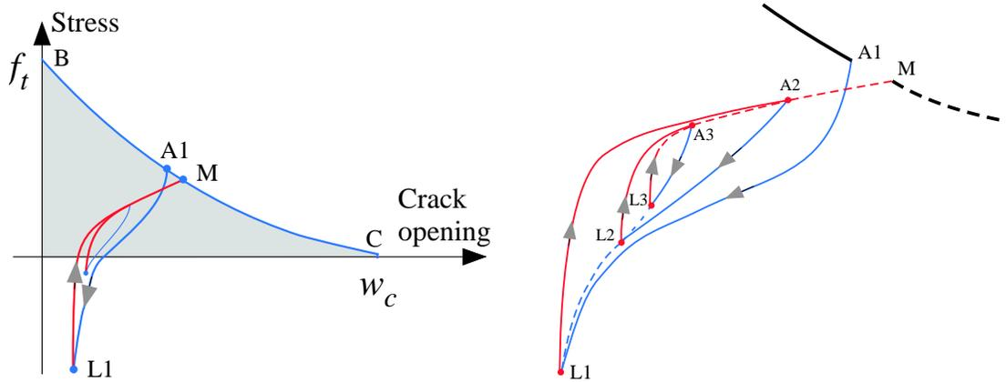
Figure 1. Cohesive stress-*COD* law (left) and hysteric unloading and reloading loop according to the Continuous Function Model (right).
