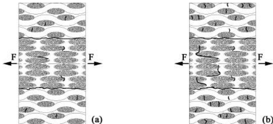
Figure 7. Damage patterns under tension-tension loading, lay-up  $[0_3/45_2]_s$ .
