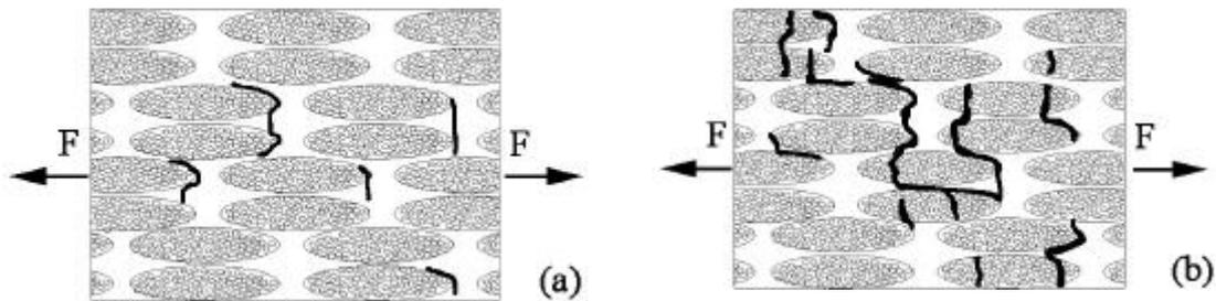
Figure 5. Damage patterns under tension-tension loading, lay-up  $[45]_{10}$ .
