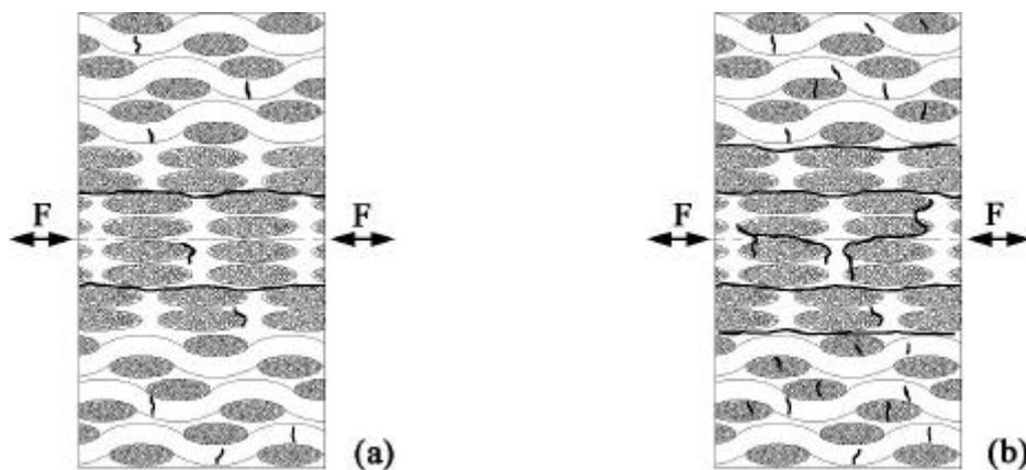
Figure 8. Damage patterns under tension-compression loading, lay-up  $[0_3/45_2]_s$ .
