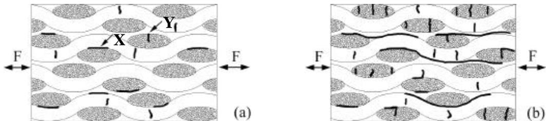
Figure 4. Damage patterns under tension-compression loading, lay-up  $[0]_{10}$ .
