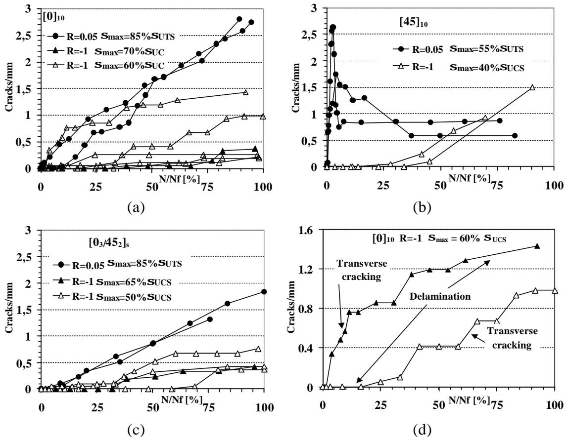
Figure 9. Crack density vs normalised fatigue life.
