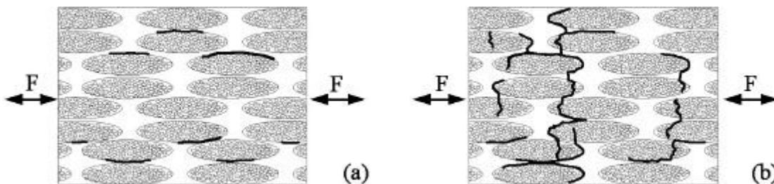
Figure 6. Damage patterns under tension-compression loading, lay-up  $[45]_{10}$ .
