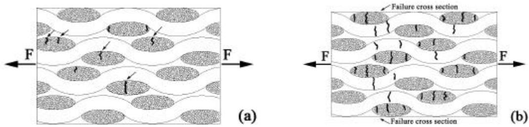
Figure 3. Damage patterns under tension-tension loading, lay-up  $[0]_{10}$ .
