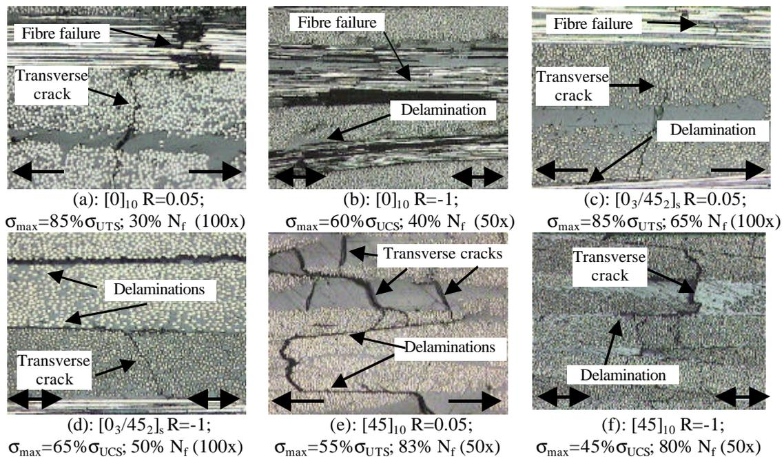
Figure 2. Microscopic observation of the main fatigue damage mechanisms.
