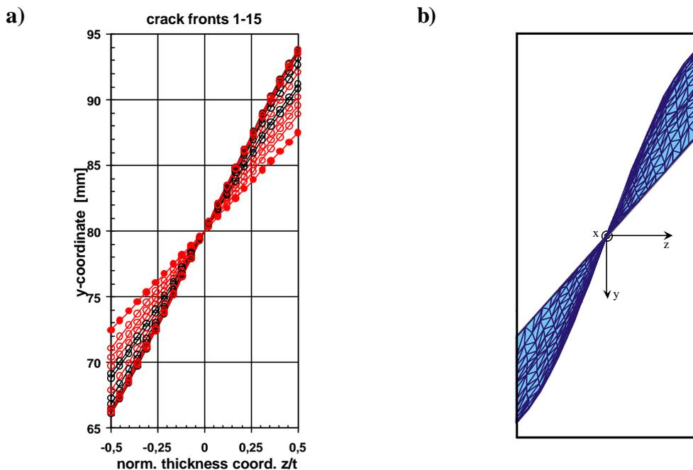
Figure 7. Development of crack fronts for simulated fatigue crack growth from initial crack (crack front 1) to final crack (crack front 15)
