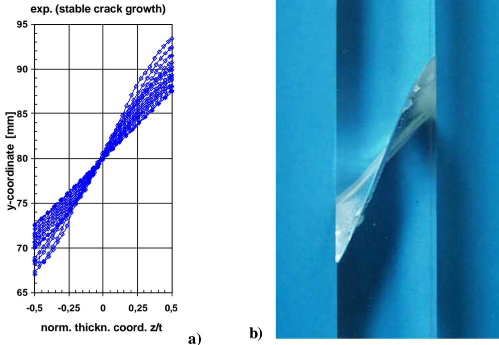
Figure 8. Development of crack fronts for stable crack growth in the experimental test specimen
