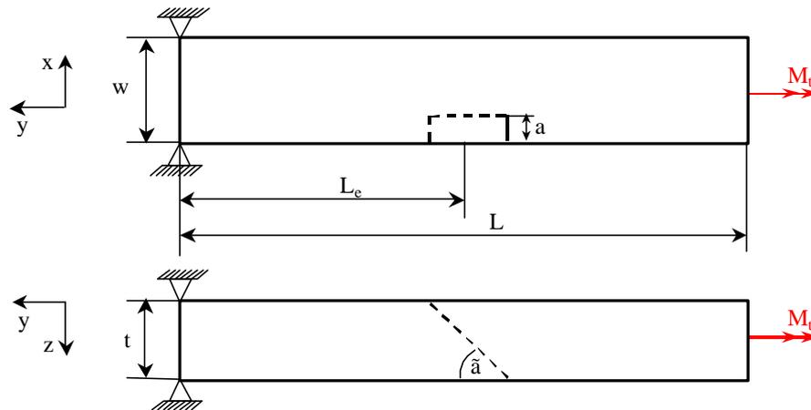
Figure 1. SEN-specimen with an inclined plane ( $\alpha=45^\circ$ ) of the initial crack or notch subject to torsion loading
