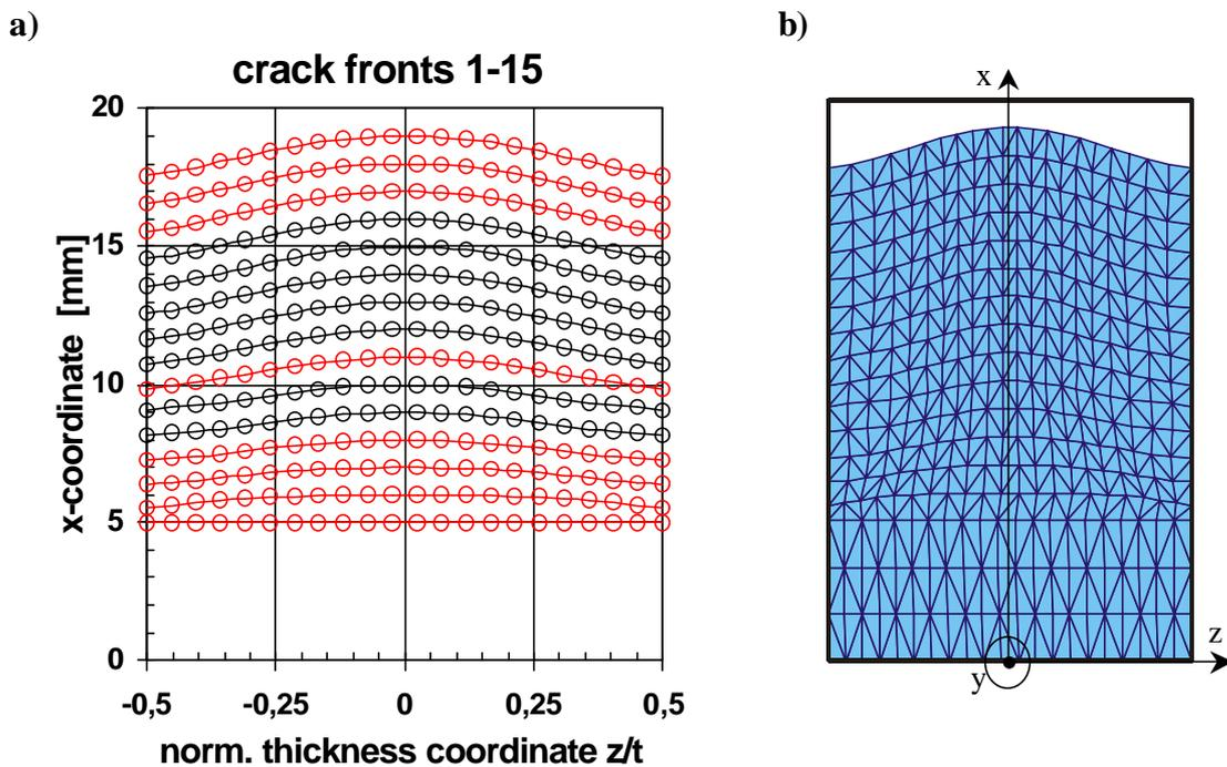
Figure 6. Development of crack fronts for simulated fatigue crack growth from initial crack (crack front 1) to final crack (crack front 15)
