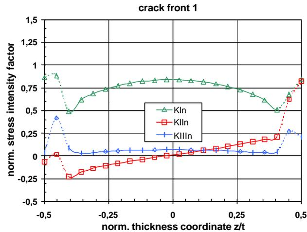
Figure 4. Norm. SIFs along the crack front for the initial inclined crack (crack front 1)
