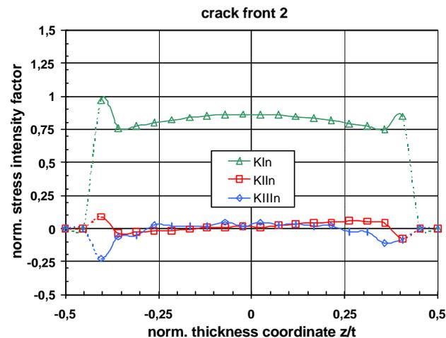
Figure 5. Norm. SIFs along the crack front after the 1<sup>st</sup> increment of computationally simulated fatigue crack growth ( $\Delta a_{\max}=1\text{mm}$ , crack front 2,  $a_{\max}=6\text{mm}$ .)
