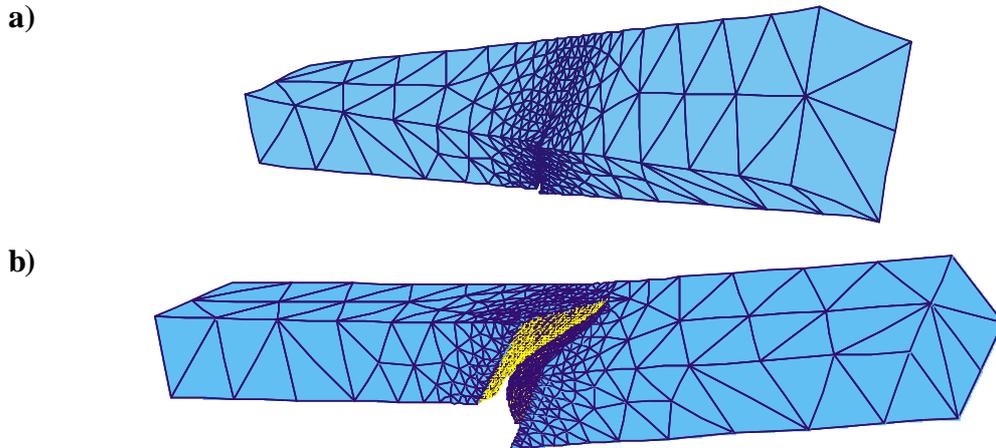
Figure 2. Deformed FE-model of the twisted SEN-specimen a) with initial crack ( $a=a_1=5\text{mm}$ ,  $g=45^\circ$ ), b) with twisted and warped crack after 14 steps of simulated incremental fatigue crack growth ( $\Delta a_{\text{max}}=1\text{mm}$ ,  $a_{\text{max}}=19\text{mm}$ , displ. magn. DMF=50)
