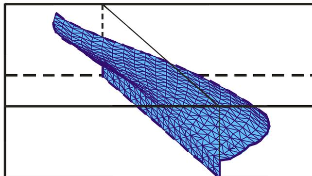
Figure 3. SEN-specimen with FE-mesh of the S-shaped crack after 14 steps of simulated incremental fatigue crack growth ( $\Delta a_{\text{max}}=1\text{mm}$ ,  $a_{\text{max}}=19\text{mm}$ )
