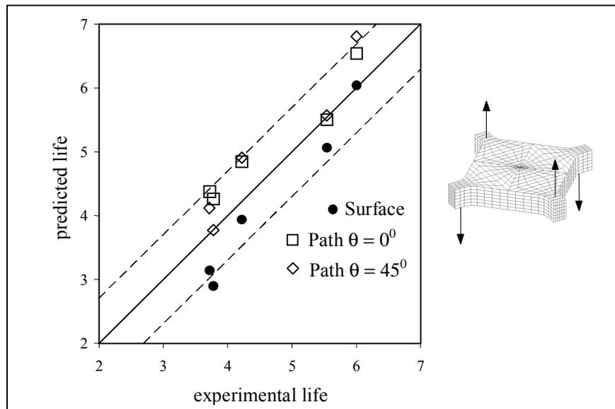
Figure 5. Experimental and predicted lives of the rhombic plate specimens using a subsurface shear strain damage parameter and two different strain paths [8].
