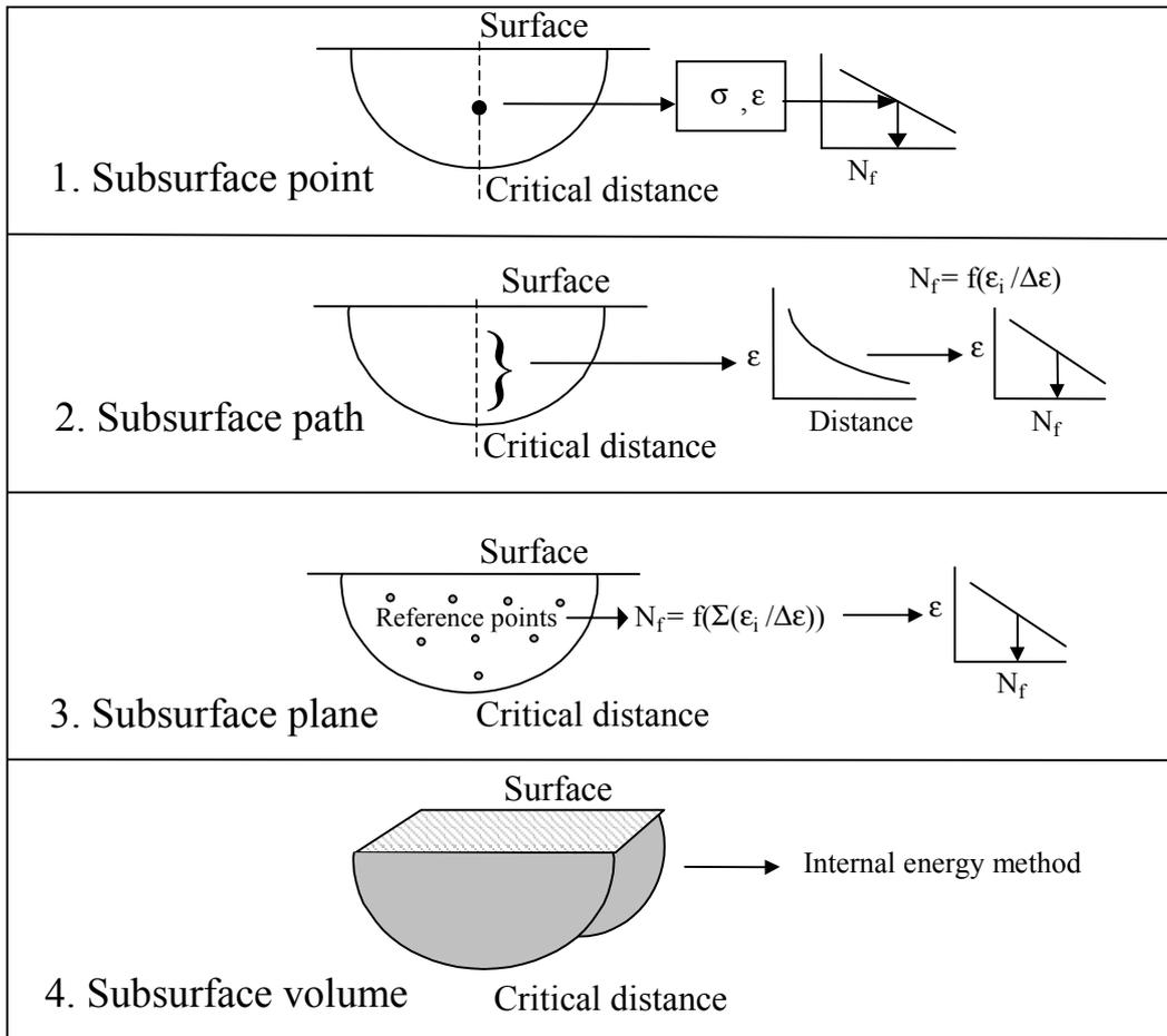
Figure 2. Illustration of subsurface fatigue model types.
