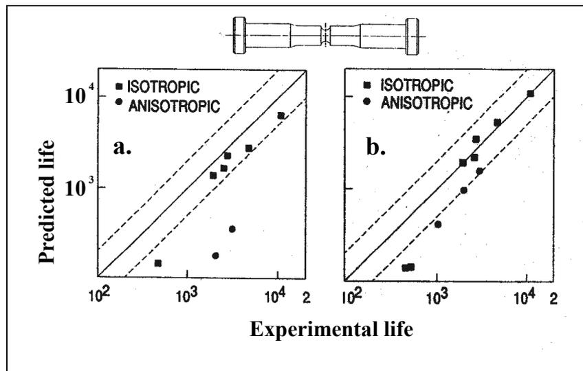
Figure 4. Predicted and experimental lives of axisymmetric notch specimens using biaxial data: a. Surface analysis and, b. Subsurface analysis [5].
