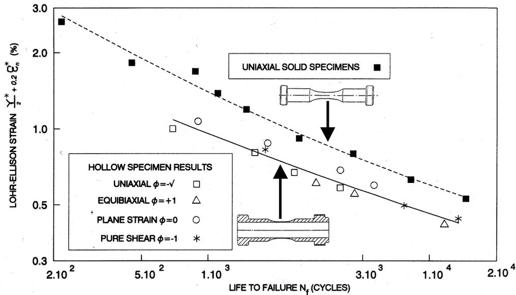
Figure 1. Fatigue lives of biaxial hollow specimens and uniaxial solid specimens [1].
