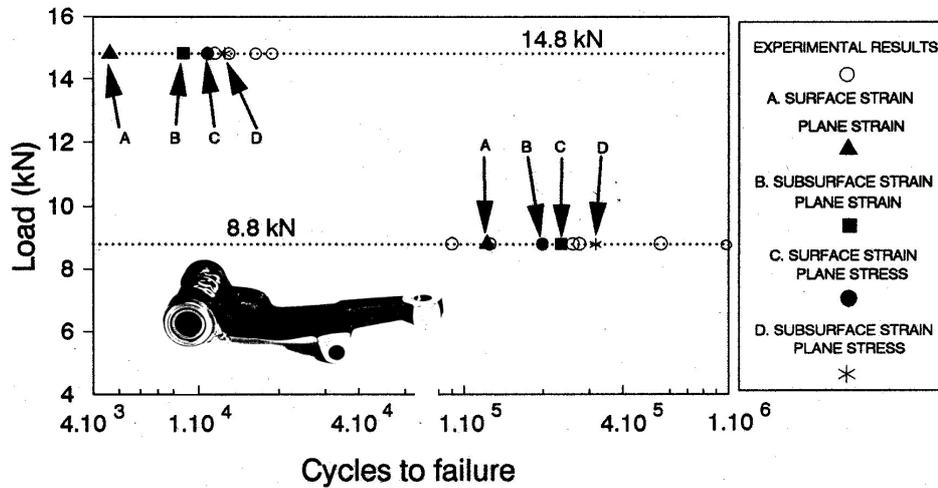
Figure 6. Experimental and predicted lives of the Metro car suspension arm [1].
