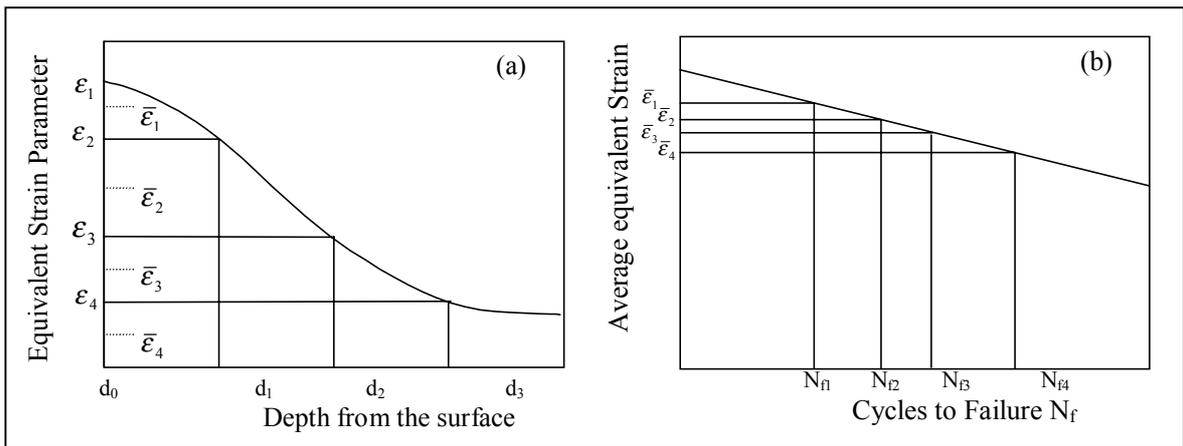
Figure 3. (a) The subsurface average strain and strain increments; (b) The predicted life to failure using the calculated average strain.
