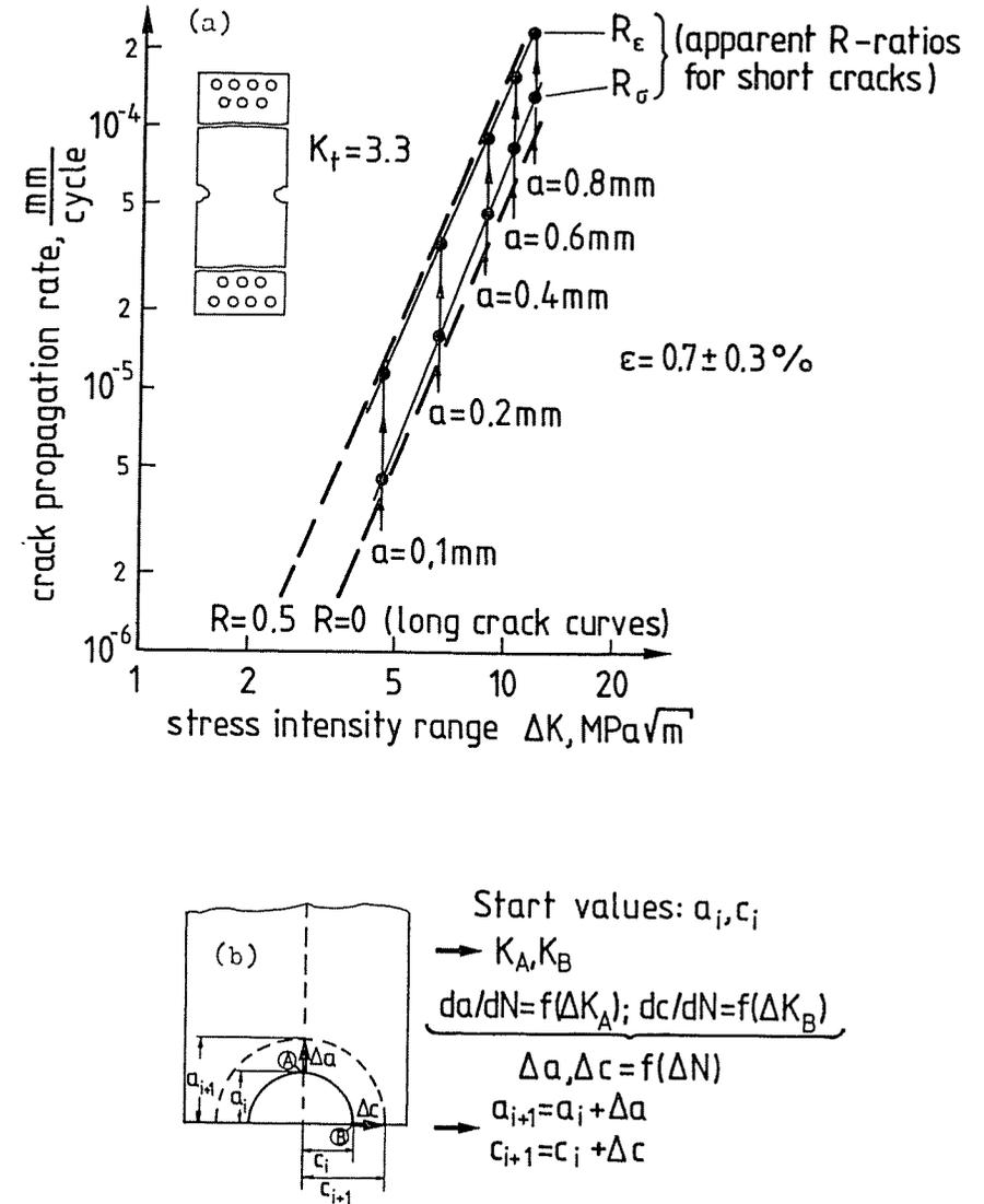
Fig 10 Crack growth prediction on the basis of the apparent  $R$  ratios,  $R_\sigma$  and  $R_\epsilon$  for short cracks. (a) Evaluation of apparent  $R$  ratios for short cracks (b) crack growth prediction (schematic)
