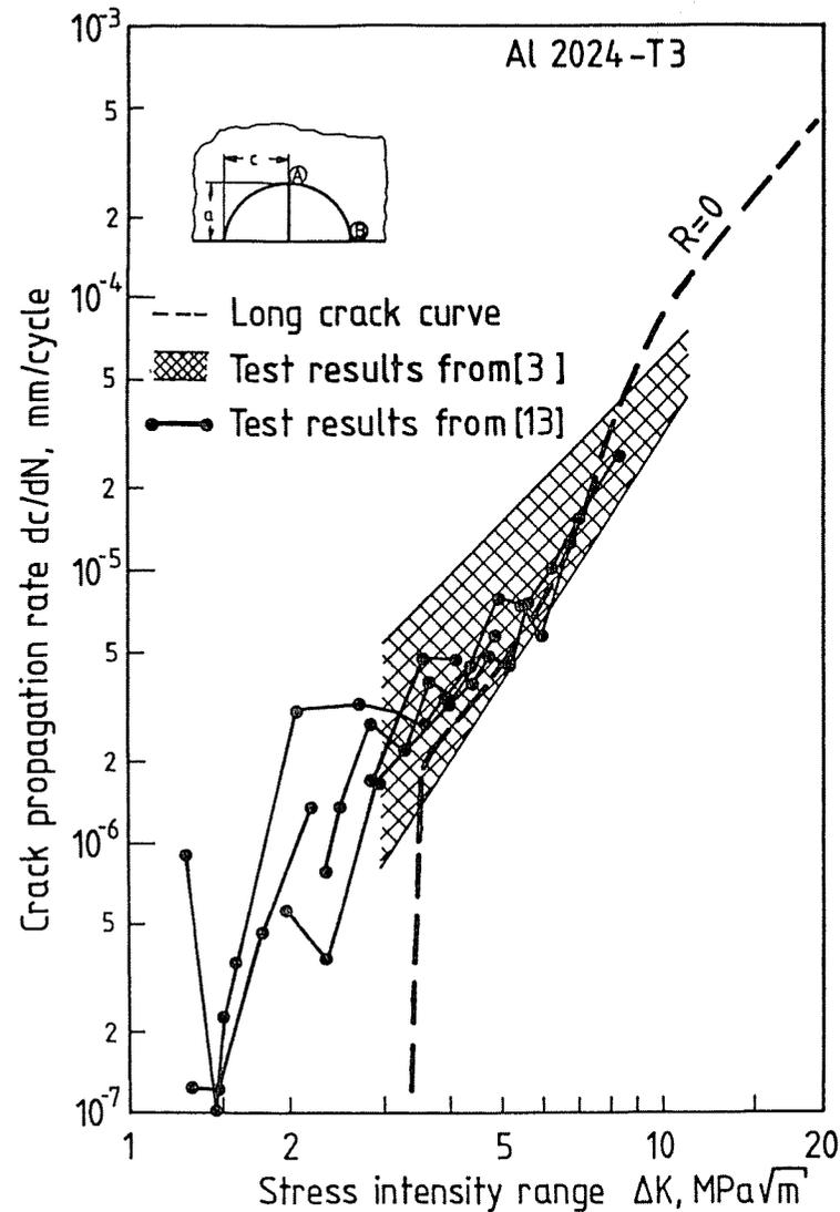
Fig 12 Representation of the behaviour of microstructurally short cracks and of mechanically short cracks in a  $dc/dN$  vs  $\Delta K$  representation
