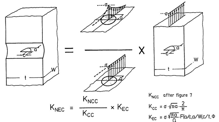
Fig 8 Similarity approach for the stress intensity factor at a notch (three-dimensional case)
