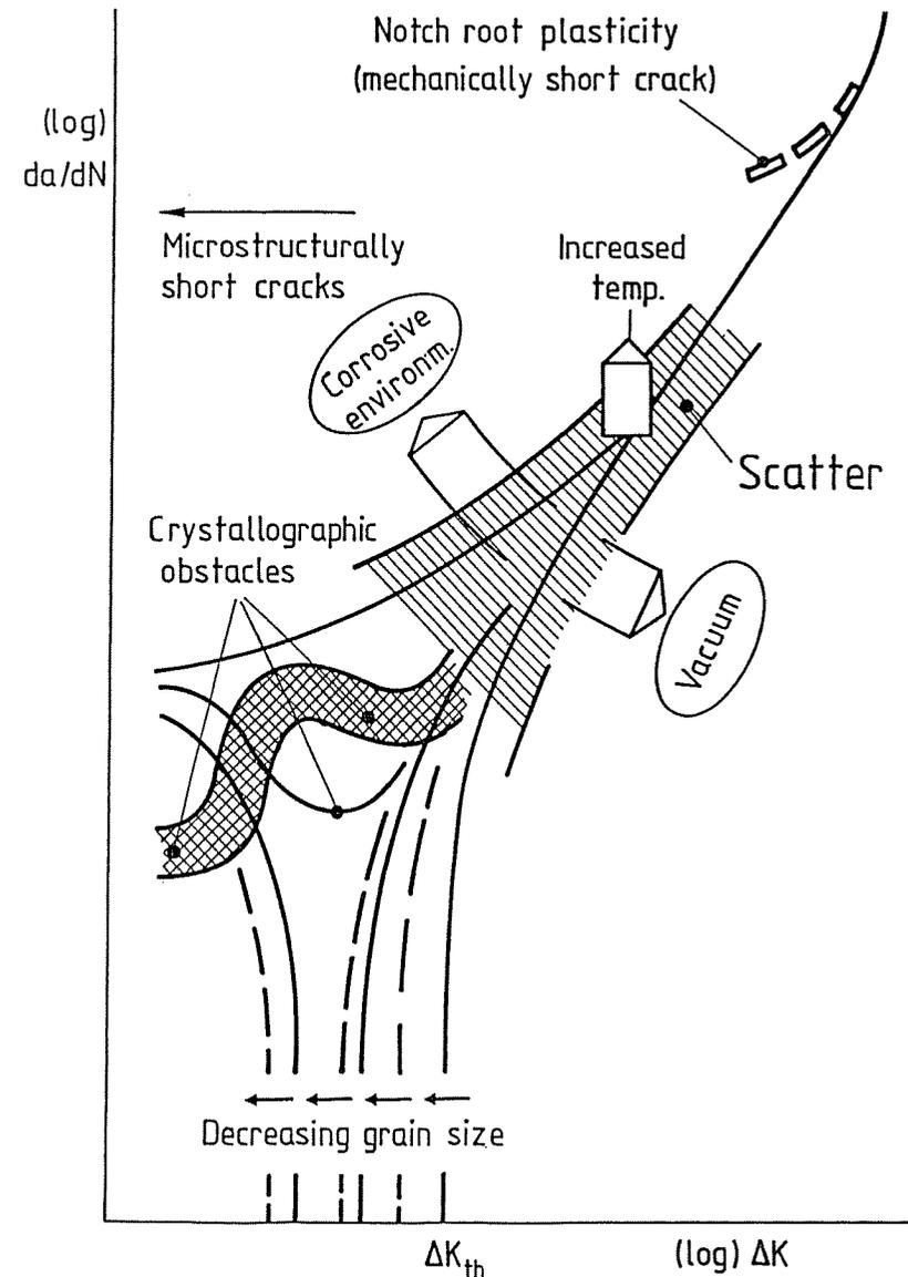
Fig 1 Characteristics of short cracks and transition to long crack behaviour
