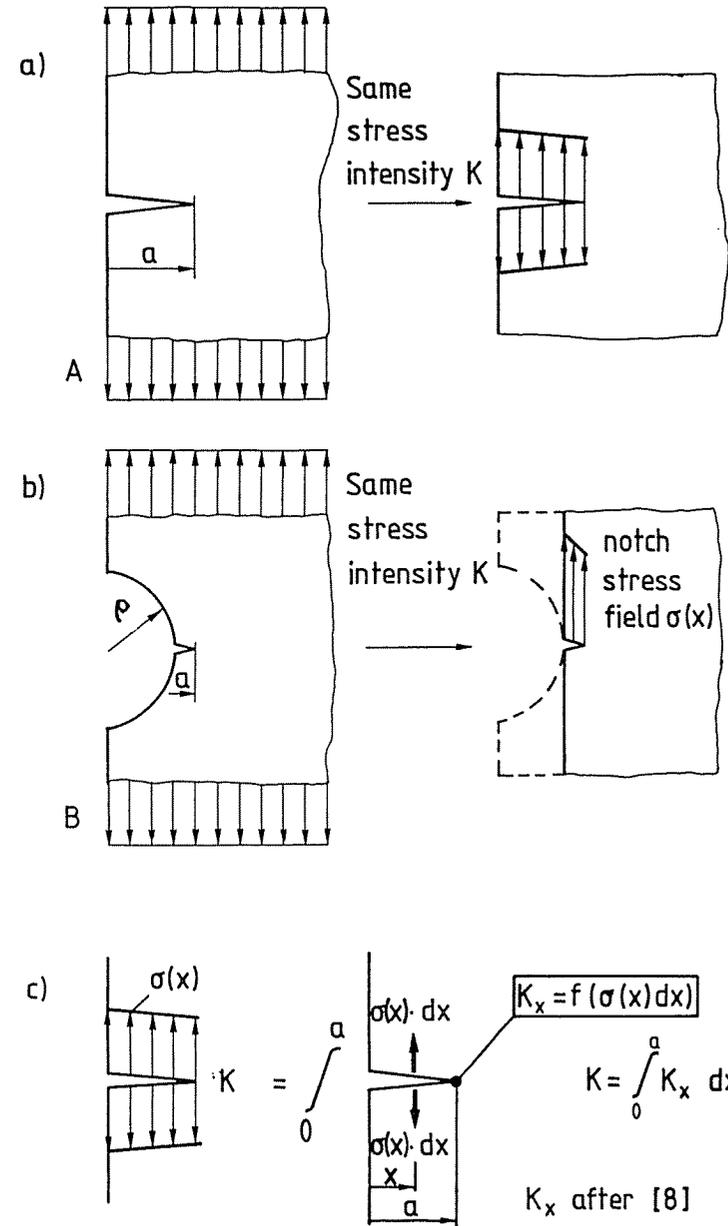
Fig 6 Evaluation of stress intensity factors in unnotched and notched configurations (two-dimensional case)
