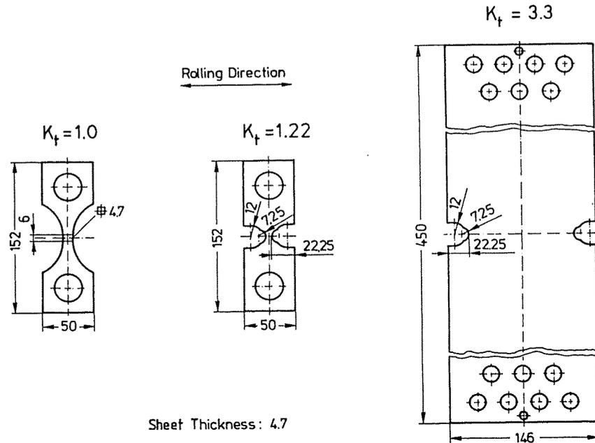
Fig 2 Specimens for the experimental investigations (dimensions in mm)
