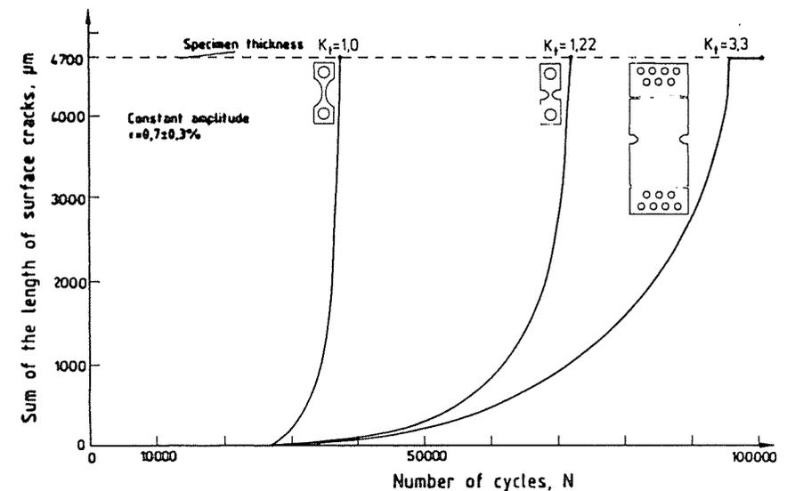
Fig 4 Crack initiation and propagation behaviour for the specimens shown in Fig. 2
