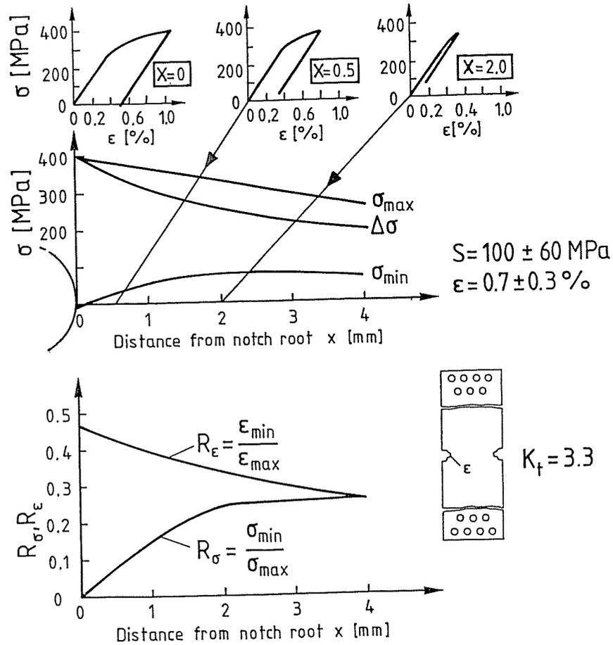
Fig 9 Behaviour of stresses and strains (without a crack) as a function of the distance from the notch for the  $K_t = 3.3$  specimen, and behaviour of the stress ratio,  $R_\sigma$ , and the strain ratio,  $R_\epsilon$
