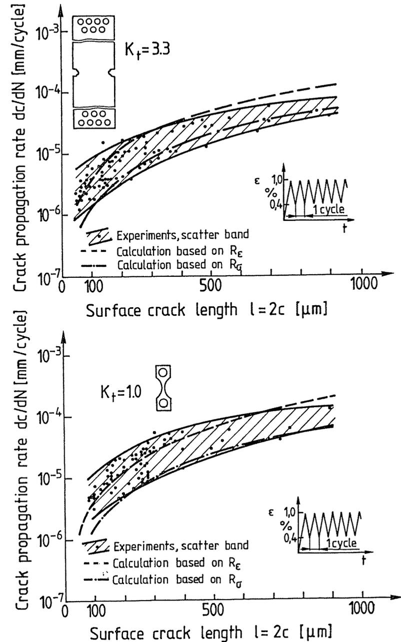
Fig. 11 Crack growth calculations based on  $R_\sigma$  and  $R_\epsilon$  for the experimental data from Fig. 5 and for the unnotched specimen in Fig. 2
