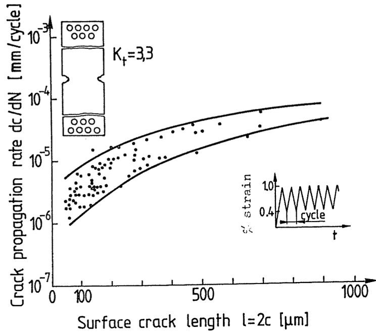
Fig 5 Scatter band of the crack propagation data as observed on the notch surface of  $K_t = 3.3$  specimens
