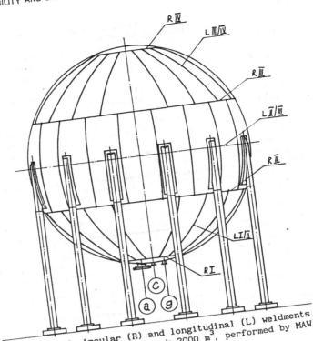
Figure 1 Scheme of circular (R) and longitudinal (L) weldments disposition on spherical storage tank 2000 m, performed by MAW
