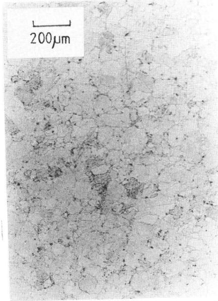
Fig.2 Necklace microstructure of polycrystalline U720
