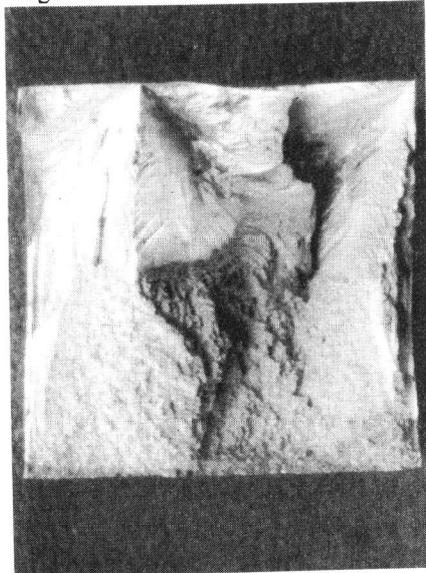
Fig.7 Crack propagation down  $\{111\}$  planes in single crystal short crack case
