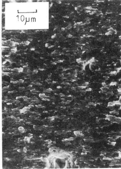
Fig.6 Non-faceted fatigue surface found in bulk of single crystal long crack case
