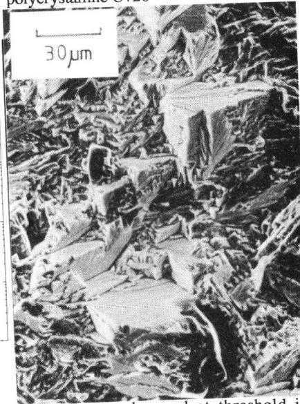
Fig.4 Facets observed at threshold in polycrystalline U720
