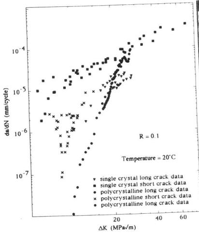
Fig.3  $da/dN$  versus  $\Delta K$  for long and short cracks in U720
