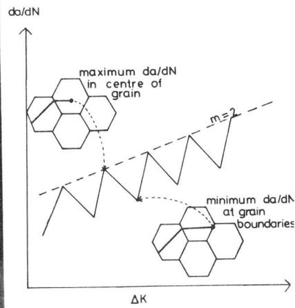
Fig.8 Schematic diagram showing typical scatter of polycrystalline short crack tests
