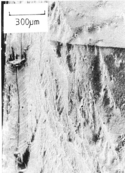
Fig.5 Side facets formed in single crystal long crack case
