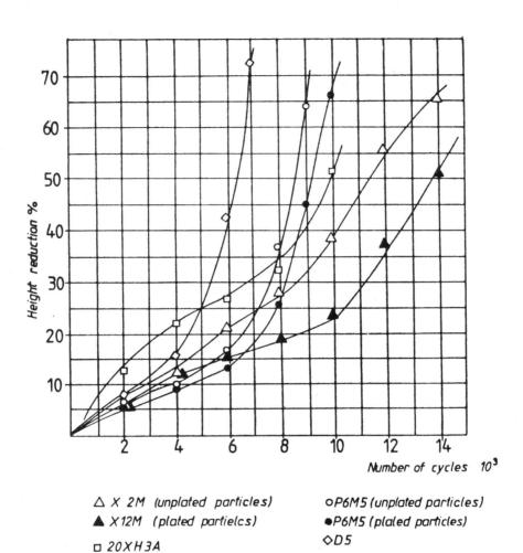
Fig.1 Resistance to impact loading of tested materials
