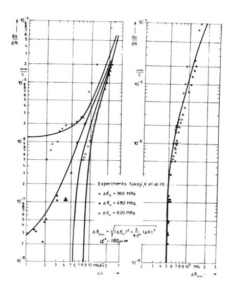
Figure 4 Propagation of small fatigue cracks in a low steel S lo C - fine grained material d= 24 m  $\,$
