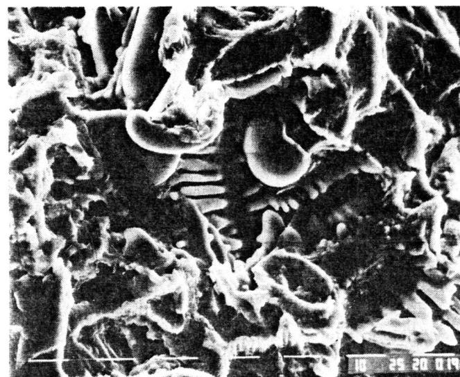
Figure 8 - Fracture across a region of porosity originated in the casting process. (1000x)
