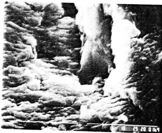
Figure 5 - Striation formation in the aluminium-rich constituent at high frequency. (5000x)
