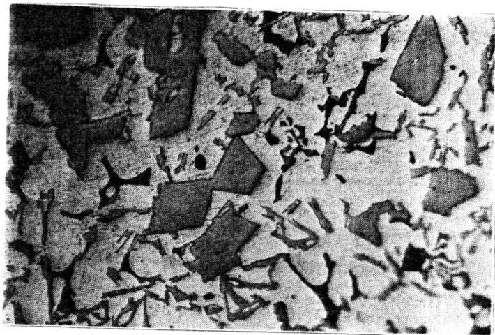
Figure 1 - Microstructure of LM-30,
