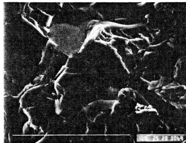
Figure 7 - Cleavage fracture of the silicon-rich constituent. (750x)
