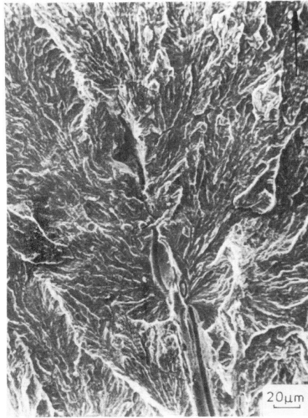
Figure 5 Brittle mode of cracking spreading from MnS inclusion
