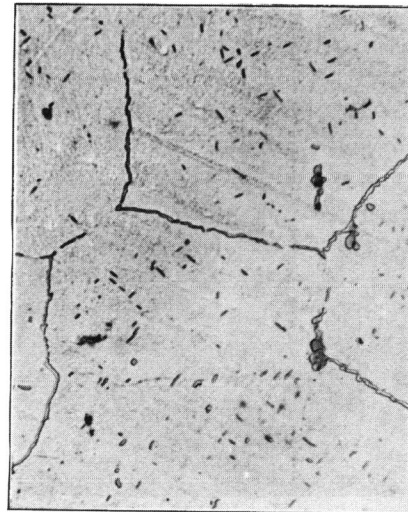
Fig. 2. Deformation structure and partly recrystallized structure.
