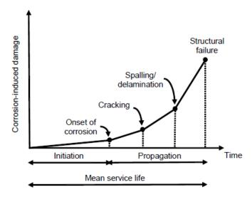
In this work, we propose a model for the time of corrosion initiation when the chloride concentration at the reinforcement level has reached the so called 'threshold value'. The length of the corrosion initiation time is controlled by the depth and quality of the concrete (permeability, cracking intensity), the presence of protective system, the rate of chloride ingress, the chloride concentration at the surface.
