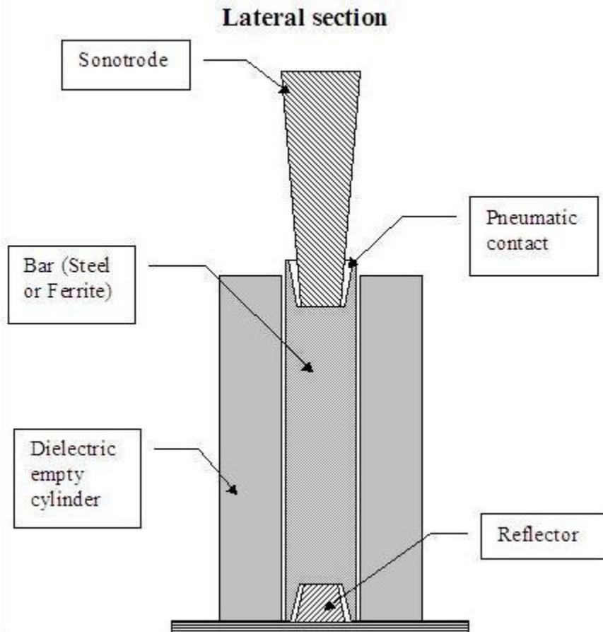
Fig 1: Experimental set-up. Lateral section.
