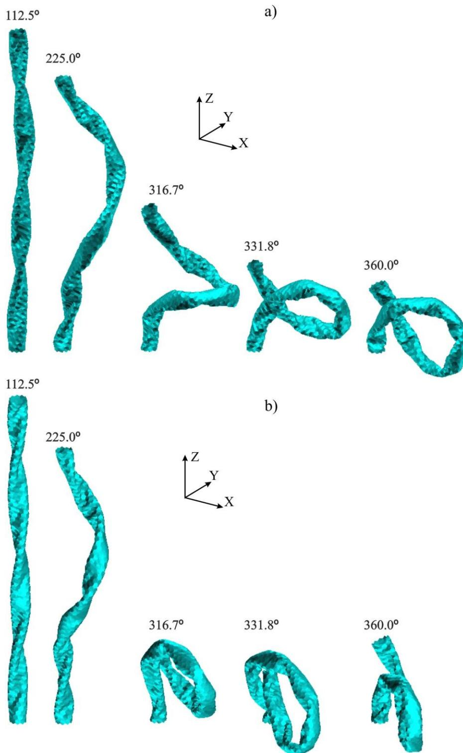
Fig. 8. Post-buckling configurations of the twisted (10,0) zigzag SWCNT under dynamic deformation for  $\dot{\varphi} = 3.6$  degr./ps (values of the twisting angle  $\varphi$  are given near the deformed configurations) obtained in solutions of the unperturbed problems using: a) the mixed MM/MSM method; b) the standard MM method.
