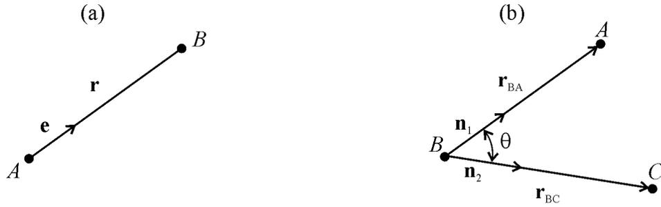
Fig. 1. Elements used to model SWCNTs: (a) two-body potential element; (b) three-body potential element.
