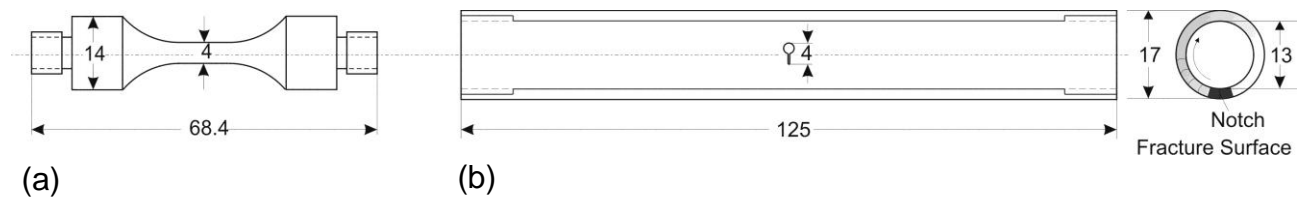
Fig. 1. Shape of (a) fatigue specimens for S-N tests and (b) tubular specimens for fatigue crack growth measurements.
