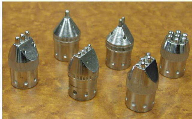
Fig.2. A set of interchangeable working heads for UIT/UP [7].
