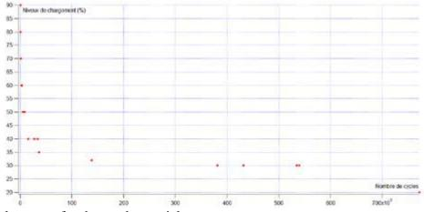
Fig.3. Wöhler curve for the used material.
