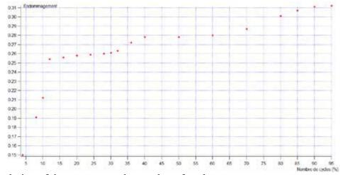
Fig.5. Evolution of damage versus the number of cycles.
