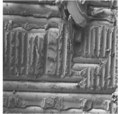
*(c) Fiber-matrix deponding* Fig.7. Observed Damage mechanisms.
