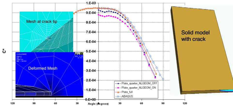
Figure 6: Surface crack in a plate: Comparison of numerical solutions ( $C^*$  units:  $N/mm.hr$ )
