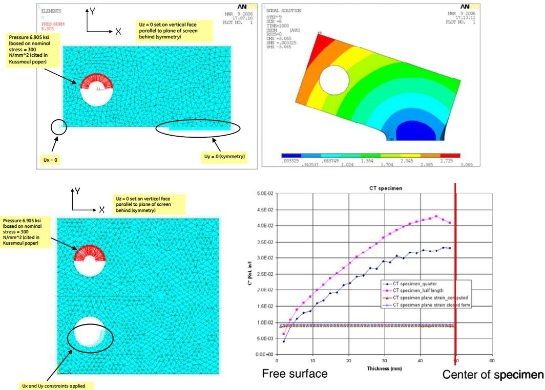
Figure 2: CT specimen – Geometry, mesh and deformed shape. Comparison of Plane strain  $C^*$  values (analytical and based on 3D computations) and through the thickness calculations is shown in chart.
