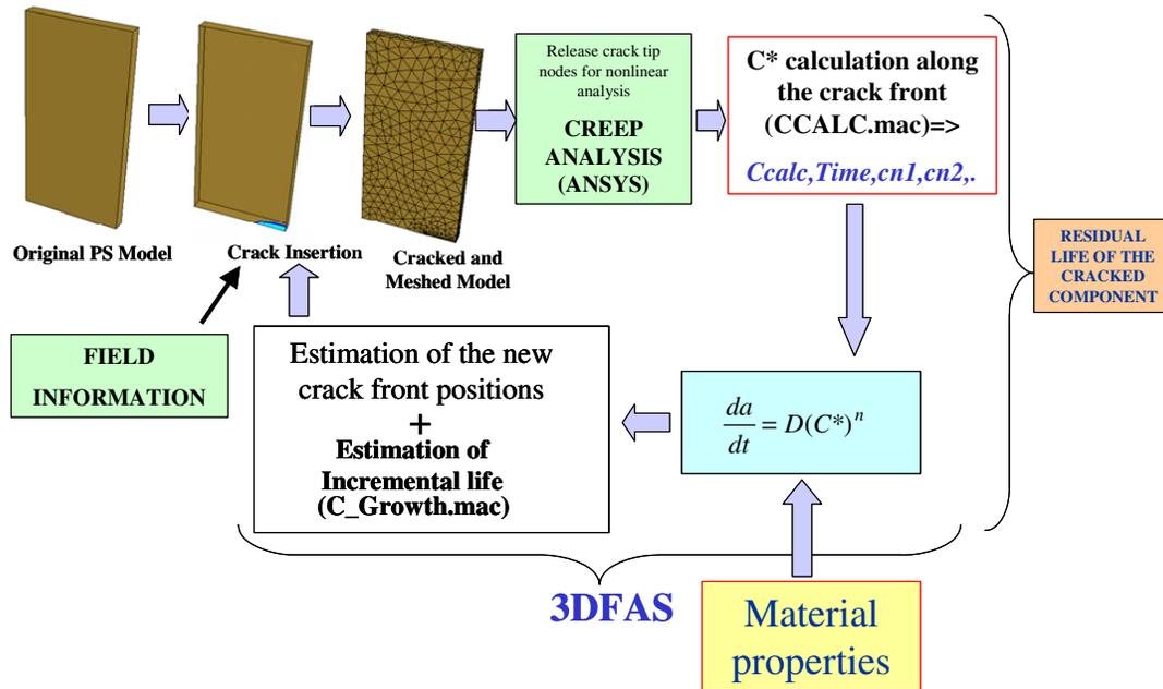
Figure 1: 3D Fracture Mechanics based Creep crack growth methodology
