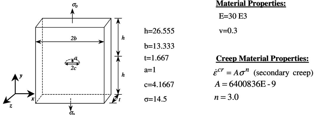
Figure 5: Schematic of surface crack geometry and values used in analysis (Note material properties used were in British units – stress (ksi), Young’s modulus (ksi), creep rate (per hour))
