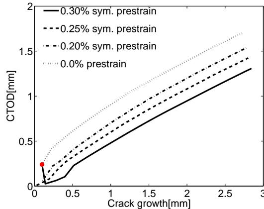
Fig. 7. Effect of prestrain history on the ductile fracture resistance of SENT specimens [15]
