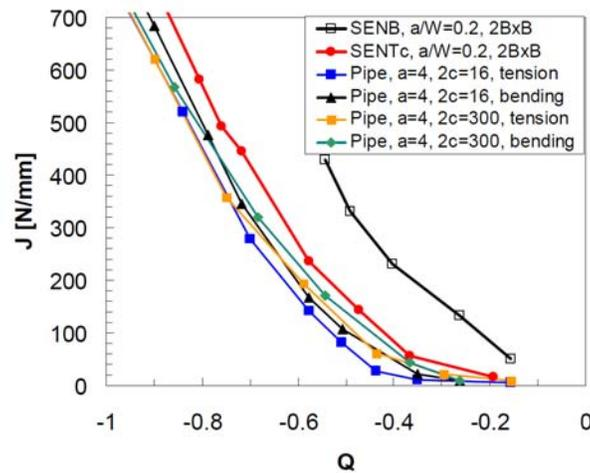
Fig. 2 Comparison of the crack tip constraint of cracked pipe models with SENT and SENB specimens [8].
