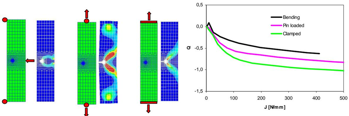
Fig. 3 Comparison of the deformation modes and crack tip constraints ( $Q$ ) of the SENB specimen with the SENT specimens with different loading conditions. Both the SENB and SENT specimens have identical geometry and crack depth.
