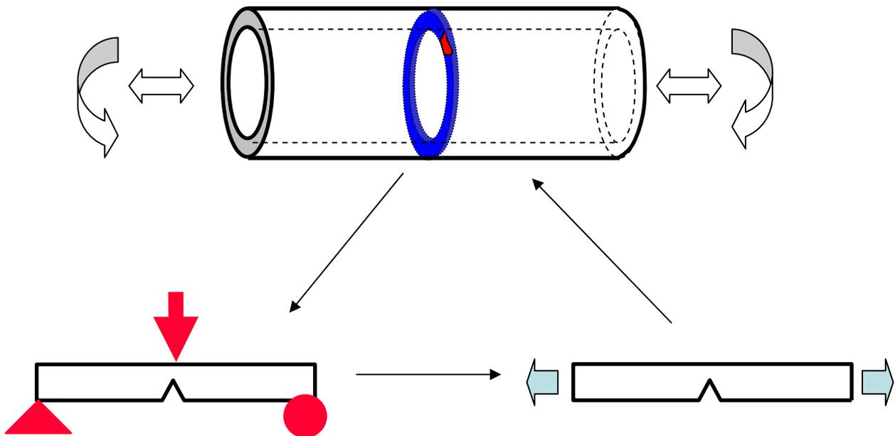
Fig. 1 Fracture mechanics testing specimens for pipeline applications: single edge notch bending specimen (SENB) versus single edge notch tension specimen (SENT).
