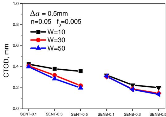
Fig. 5 Effect of specimen width ( $W$ ) and crack depth ( $a/W$ ) on the critical CTOD at 0.5 mm crack growth [14].
