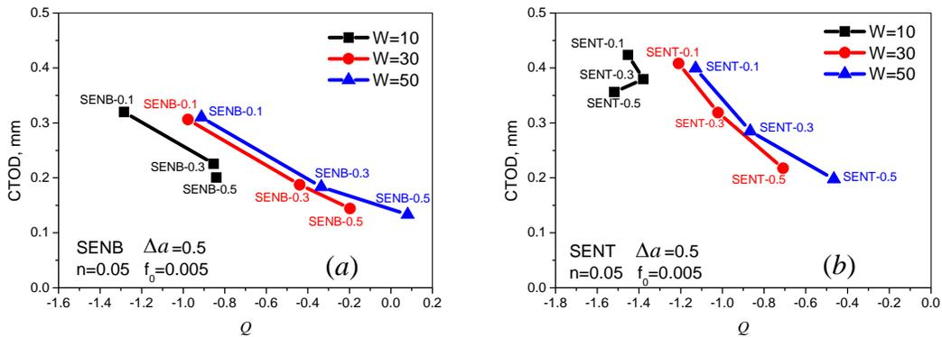
Fig. 6. CTOD- $Q$  relations for SENB and SENT specimens [14].  $a$  is the crack depth,  $W$  the specimen width,  $f_0$  the initial void volume fraction and  $n$  the power hardening exponent. SENT-0.1 indicates that a SENT specimen with  $a/W=0.1$ .
