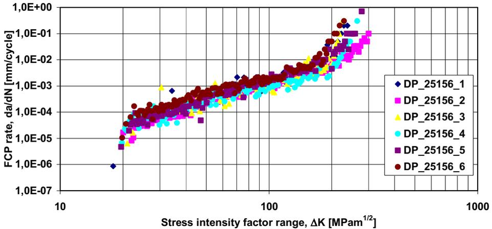
Figure 2. Kinetic diagrams of fatigue crack propagation from tested DP-25156 SENT specimens.
