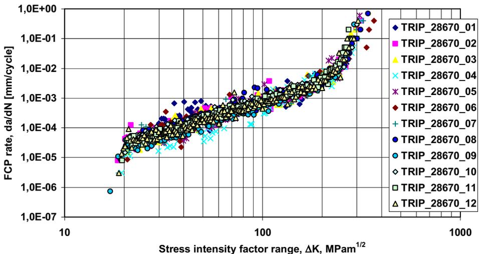
Figure 3. Kinetic diagrams of fatigue crack propagation from tested TRIP-28670 SENT specimens.
