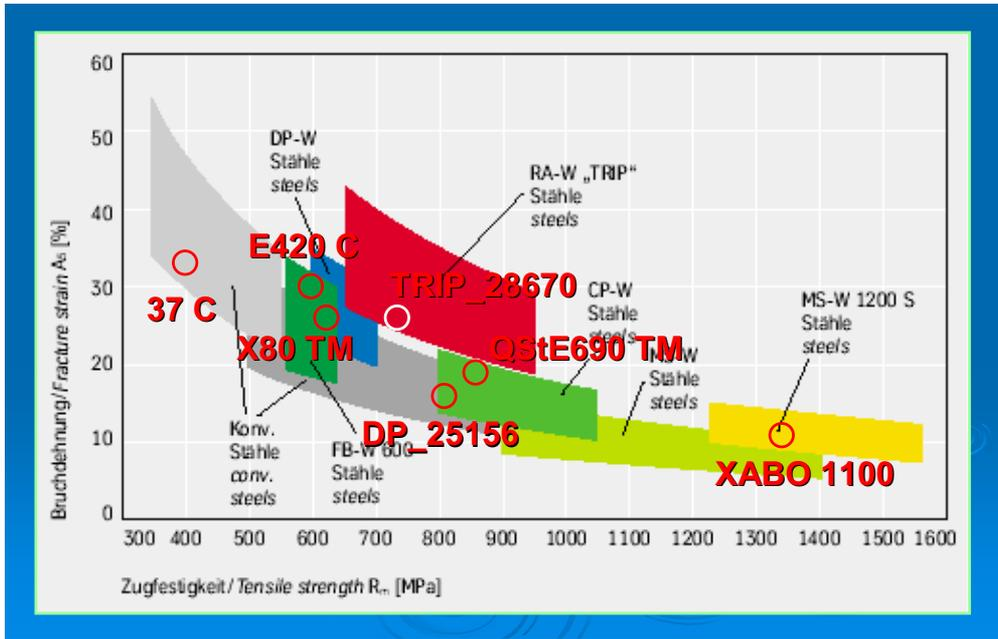
**Figure 1.** Relation between tensile strength and fracture strain for the investigated base materials.
