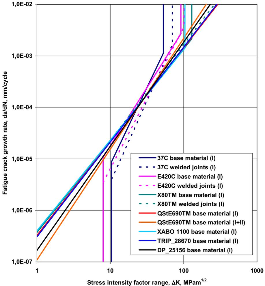
**Figure 4.** Fatigue design limit curves for micro-alloyed and HSLA steels, and their welded joints.
