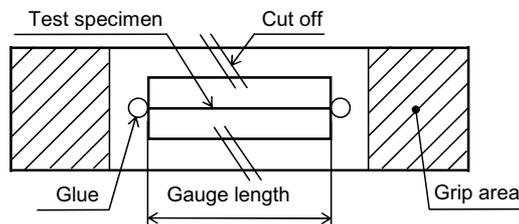
Fig. 3 Monofilament testing tab for tensile and fatigue tests.
