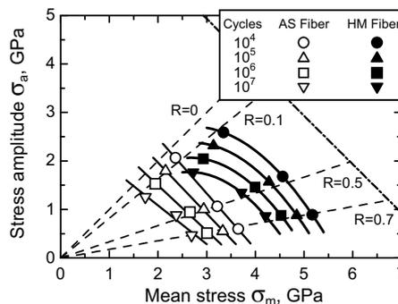
Fig. 8  $\sigma_a$ - $\sigma_m$  curves of HM and AS fibers.
