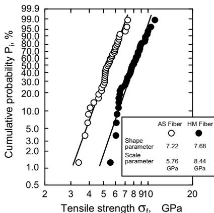
Fig. 4 Weibull distributions of tensile strength of HM and AS fibers.
