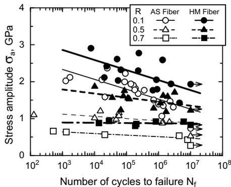
Fig. 6 S-N curves plotted stress amplitude in ordinate for HM and AS fibers.
