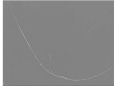
(b) Fatigue fracture with multiple splitting in a PBO fiber.
