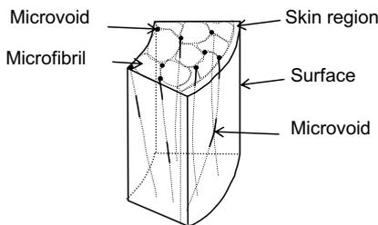
Fig. 5 Schematic illustration of internal structure of PBO fiber.
