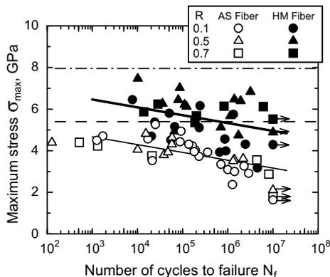
Fig. 7 S-N curves plotted maximum stress in ordinate for HM and AS fibers.
