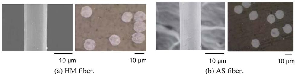
Fig. 2 Surfaces and cross sectional areas of two types of PBO fiber.
