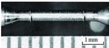
Fig. 2. Photograph of miniature creep specimen
