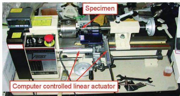
Fig. 3. Computer controlled desktop type precision lathe
