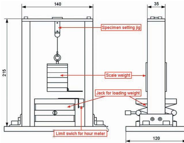
Fig. 4. Assembly drawing of miniature creep testing equipment
