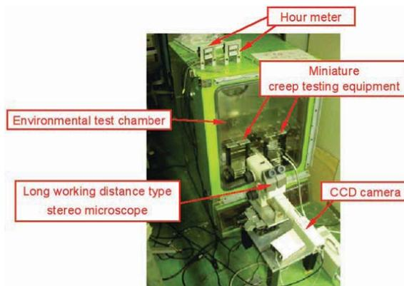
Fig. 5. Whole view of creep testing system
