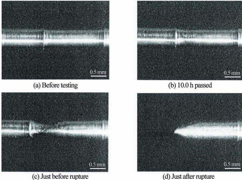
Fig. 8. Example of series photographs of deformed miniature specimen ( $\sigma = 15$  MPa,  $t_r = 16.1$  h)
