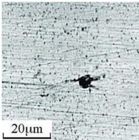
Fig. 12. Example of defect in solder
