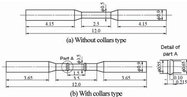
Fig. 1. Shapes and dimensions of miniature creep specimen
