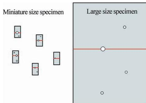
Fig. 14. Schematic illustration for defect size effects on both size specimen
