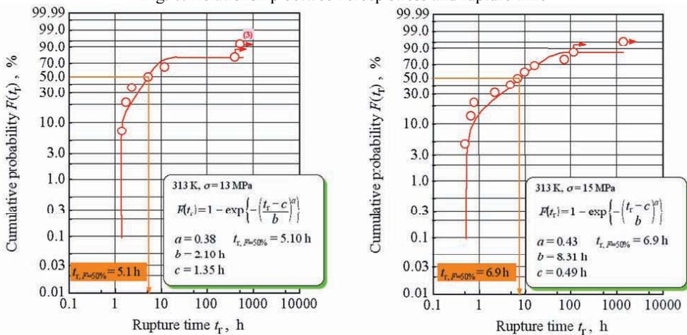
Fig. 7. Probability distributions of creep rupture time (Weibull probability graph)
