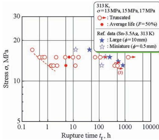
Fig. 6. Relationship between creep stress and rupture time
