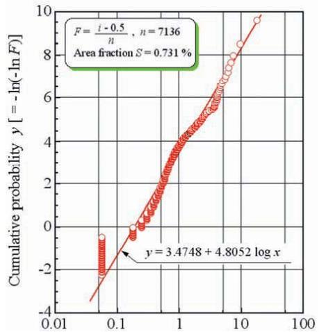
Fig. 13. Defects size distribution
