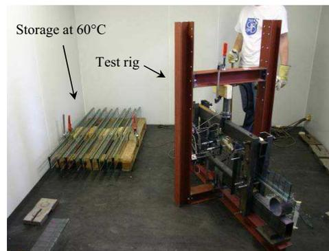
Figures 3 and 4: Beam specimens stored and tested at 60°C in a climatic room.
