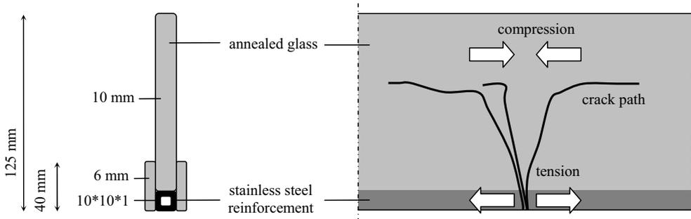
Figure 2: Left: cross-section of 1.5 m glass beam specimens; Right: post-breakage behaviour.
