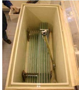
Figures 5 and 6: Beam specimens stored for 8 weeks in a salt-water-spraying container.
