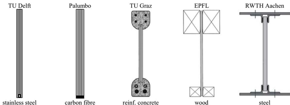
Figure 1: Different composite glass beam solutions aim for ductility at the post-failure stage.
