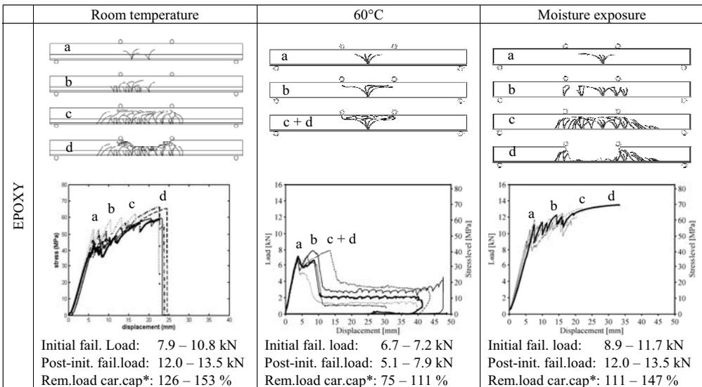
failure stages; a = initial failure, b = additional cracking, c = horizontal crack propagation, d = ultimate failure
