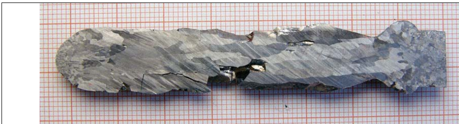
Figure 12 Fe-40-3Ti materials that was grown by the seedless floating method with growth rate 10 mm/h. The grain boundaries parallel to the growth direction are very stable in this material. Some grains were broken out during preparation of the cross-cut. The growth started at the right hand side.
