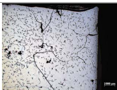
Figure 2 Microstructure of the cross-cut of the rolled sample Fe-40Al-1C. Optical microscopy.
