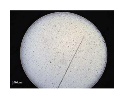
Figure 7 Fe-40Al-1C, the monocrystal prepared by the Bridgman method with the growth rate of 9 mm/h.
