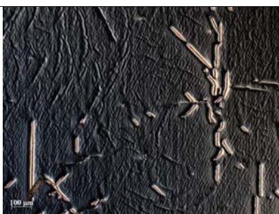
Figure 4 Detail from optical microscope showing the cracks nucleating at the interfaces of precipitates and matrix in the monocrystal Fe-40Al-1C grown by the Bridgman method.
