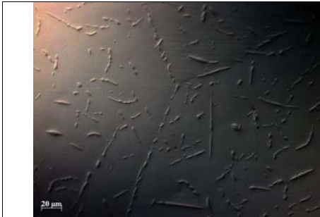
Figure 10 The as-cast material Fe-40Al-1C solidified under the ultrasound power of 800W.
