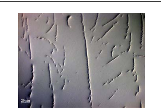
Figure 8 Detail of Fig. 7 shows the Fe 3 AlC rectangular precipitates connected into the rounded or straight patterns.
