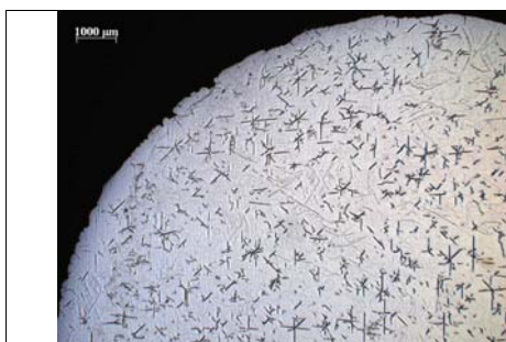
Figure 3 Asterisk cracks and \text{Fe}_3\text{AlC} precipitates in the monocrystal Fe-40Al-1C grown by the Bridgman method.
