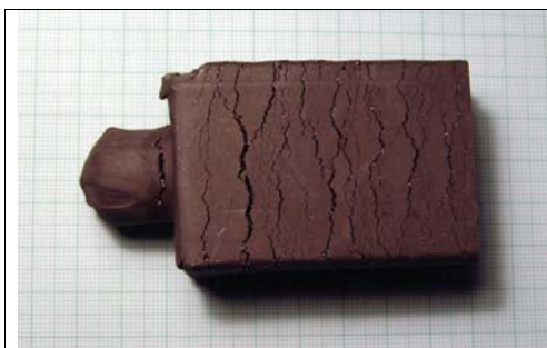
Figure 1 The Fe-40Al-1C chill cast ingot after an attempt to roll contains massive intercrystalline cracks.
