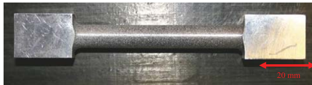
Figure 3: Prepared tensile specimen
