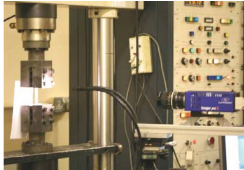
Figure 4: Experimental set-up for tensile tests
