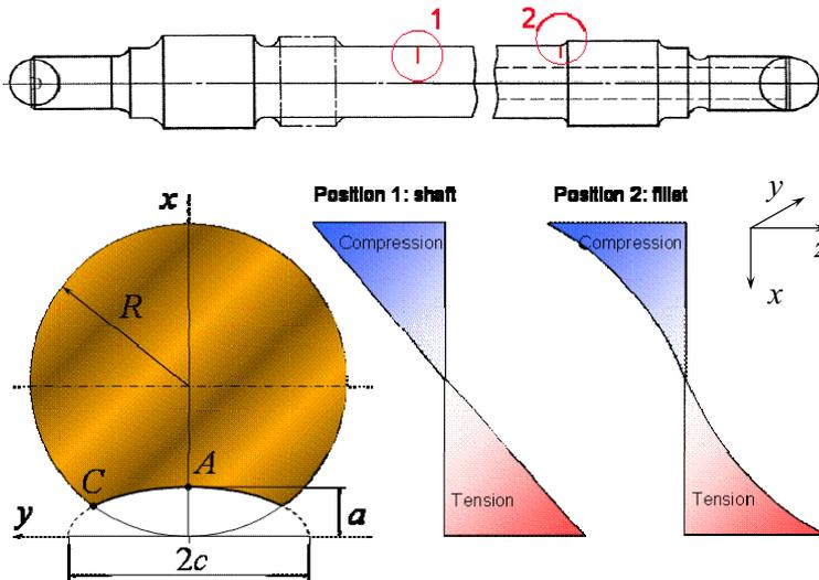
Figure 2: Schematic representation of the reference axle and stress distribution at selected cross-sections.
