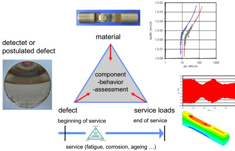
Figure 1: Fracture mechanics assessment concept.
