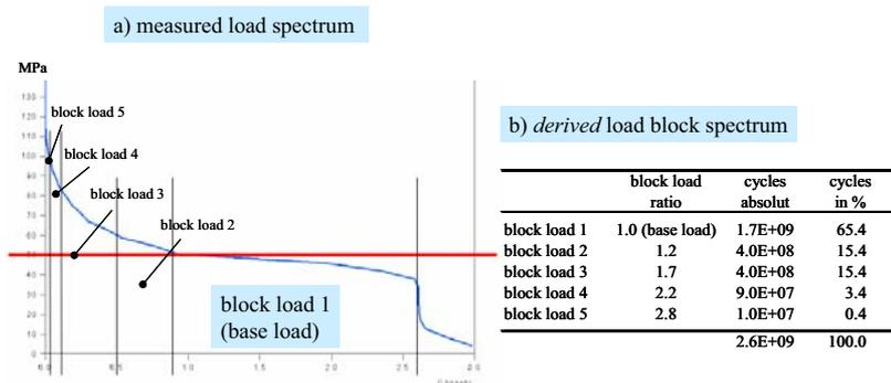
**Figure 5:** Measured load and *derived* load block spectrum.
