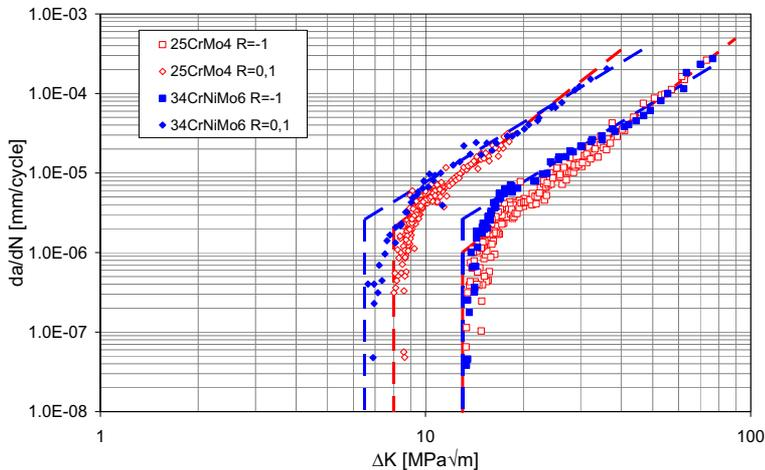
**Figure 3:** Comparison of crack propagation data of 25CrMo4 and 34CrNiMo6 at  $R=-1$  and  $R=0.1$ .
