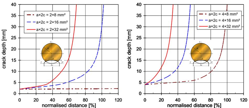
**Figure 8:** Normalised fatigue lives for different initial flaws in the shaft (here 100% fatigue life corresponds to the initial crack size of  $a \times 2c = 4 \times 8 \text{ mm}^2$ ).
