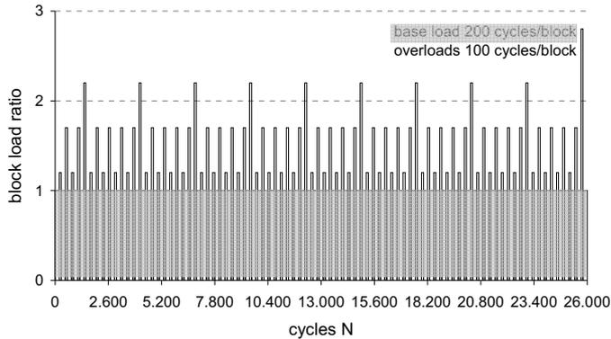
**Figure 6:** *Reduced* block load spectrum.
