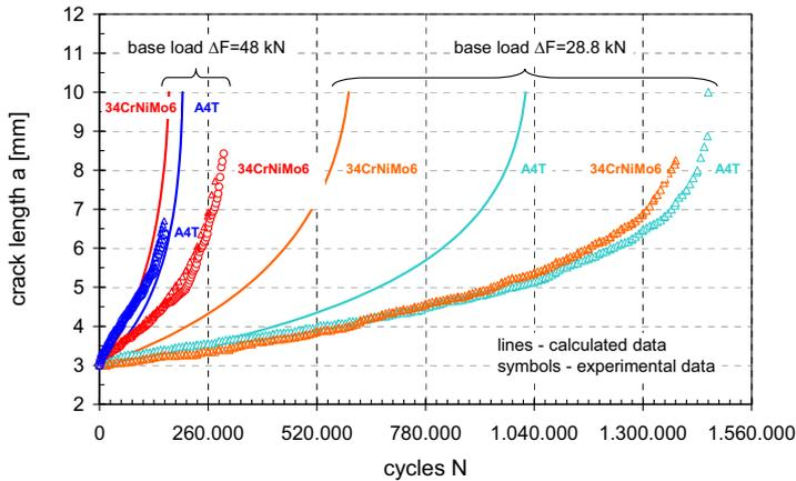
**Figure 7:** Crack propagation of 25CrMo4 (A4T) and 34CrNiMo6 axle steels under variable amplitude loading (reduced block loading) determined with M(T) specimens.
