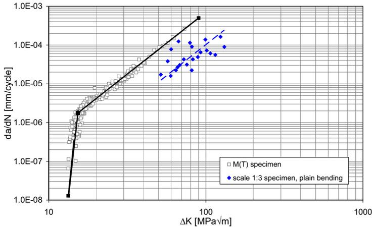
**Figure 4:** Comparison of crack propagation rates determined for M(T)-specimens and scale 1:3 component-like specimens under fully reversed loading,  $R = -1$ .
