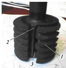
Figure 2. High temperature chamber - upper tool fork, 1- tool body with sealing grooves, 2 - bolt retainer, 3 - hole for bolt without head
