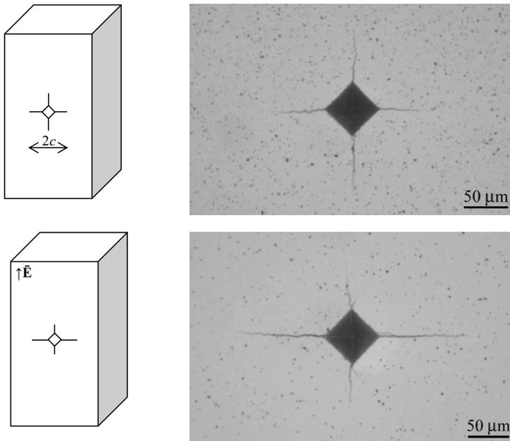
**Figure 1.** Indentation cracks parallel and perpendicular to the longitudinal direction in a) non-poled specimens and b) poled specimens, before the thermo-mechanical tests.
