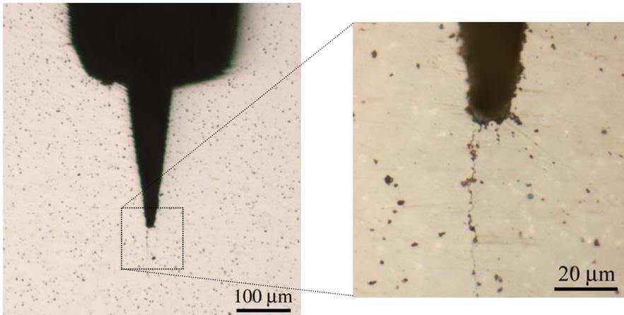
**Figure 2.** Pre-notched PZT bulk specimen for fracture toughness determination. A crack has developed during the notching process, yielding a single edge pre-crack beam (SEPB) configuration.
