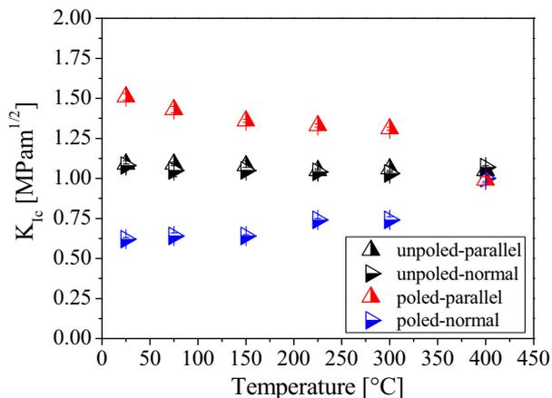
**Figure 3.** Crack growth resistance measured in poled and non-poled PZT specimens as a function of temperature. Whereas the fracture toughness remains constant and isotropic (i.e. same crack length parallel and normal to the longitudinal axis) in the non-poled specimens after the testing temperatures, an effect of the temperature in the toughness of the poled specimens can be appreciated, leading to partly depolarisation.
