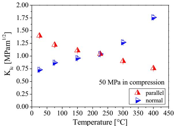
**Figure 5.** Crack growth resistance measured in poled PZT specimens after a mechanical stress of -50 MPa (compression) as a function of temperature. The mechanical stress applied against the direction of poling yield a significant depolarisation effect even at low temperatures. The crack growth resistance of the PZT reverses already for temperatures above 225 °C, reaching values up to 1.75 MPam<sup>1/2</sup> for 400 °C.
