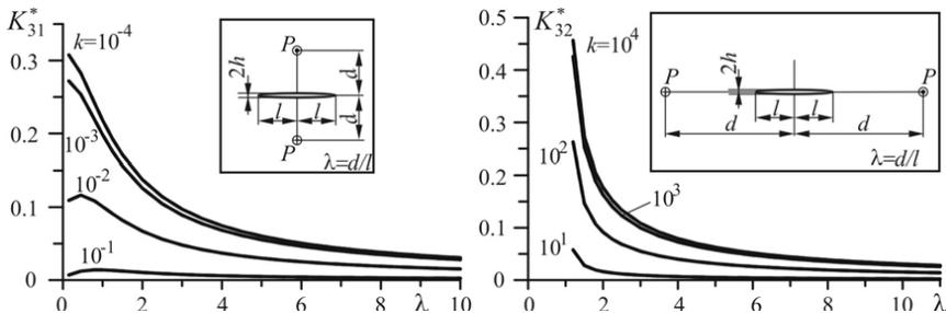
Fig. 3. GSIFs for antiplane shear of a solid with ribbon-like inclusion
