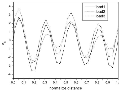
Figure 9: Distribution of shear stresses along inner microvoid edge
