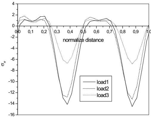
Figure 7: Distribution of radial stresses along inner microvoid edge
