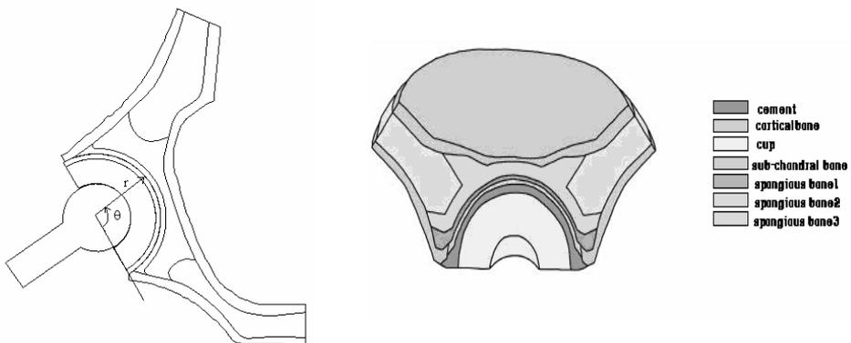
Figure 1: Cylindrical coordinate system  $(r, \theta)$ . Figure 2: Composition of a reconstructed acetabulum.
