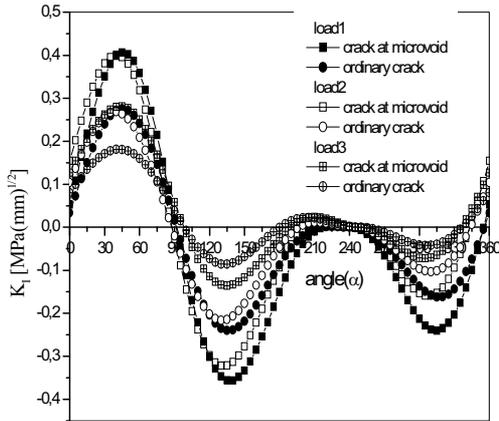
Figure12: Comparison of the  $K_I$  between the tow cracks.
