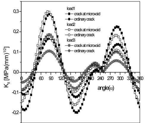
Figure13: Comparison of the  $K_{II}$  between the tow cracks.
