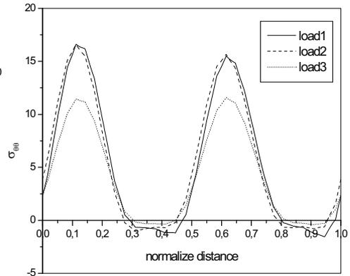
Figure 8: Distribution of circumferential stresses along inner microvoid edge
