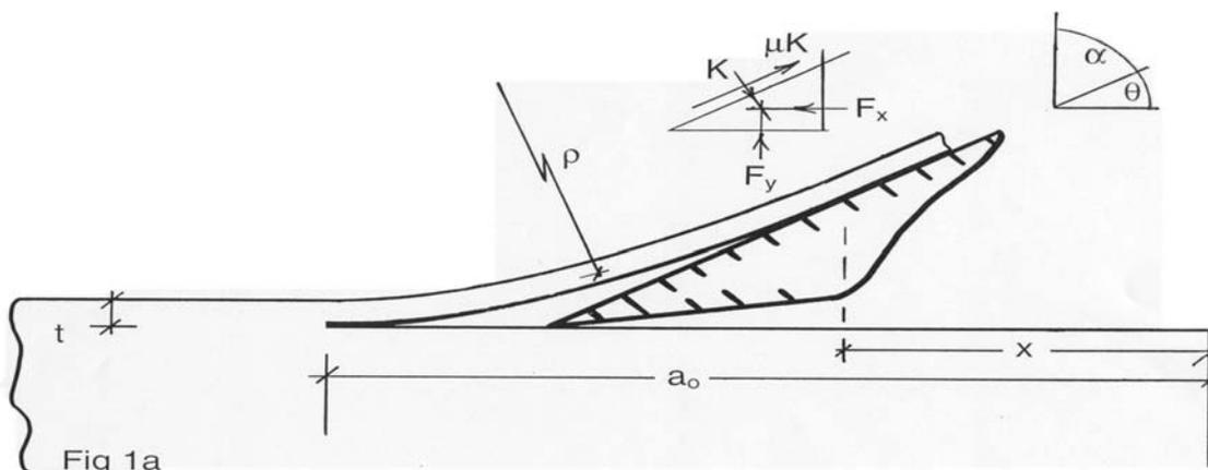
The forces on the wedge parallel and perpendicular to the cut surface are  $F_x$  and  $F_y$ . Equilibrium gives
